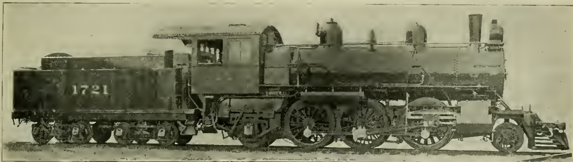
Six-Coupled Freight Locomotive, 2-6-2 Type. — Chicago, Burlington & Quincy Railway.
