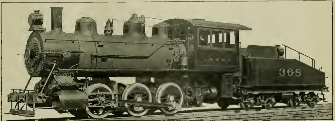
Six-Coupled Switching Locomotive with Piston Valves and Narrow Firebox. Lake Shore & Michigan Southern Railway.
