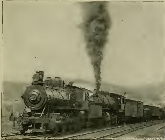
Showing Contrast Between Fuel Oil and Coal. Both Engines Are Working Hard Up Grade Entering Tunnel. This is a Fair Representation of the Results as to Smokelessness of Oil.
