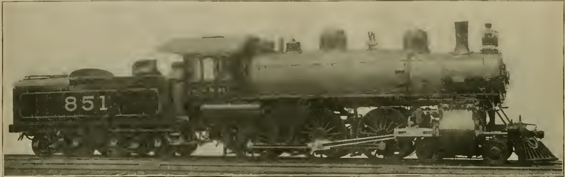
Two-Cylinder Compound Ten-Wheel Locomotive.—Canadian Pacific Railway.
