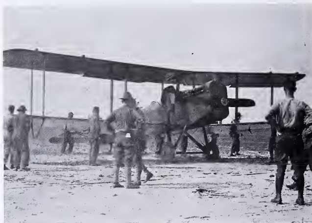
Final preparations. Note the large ground crew assisting the take off. Ignition by manually spinning the propeller was extremely hazardous.
