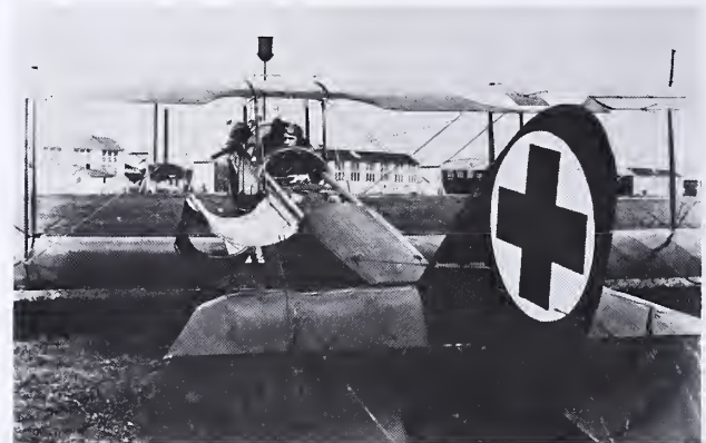
The injured, carried in a semi-reclining position, rode protected in the rear of the airplane. The modified Jenny was somewhat tail heavy.
