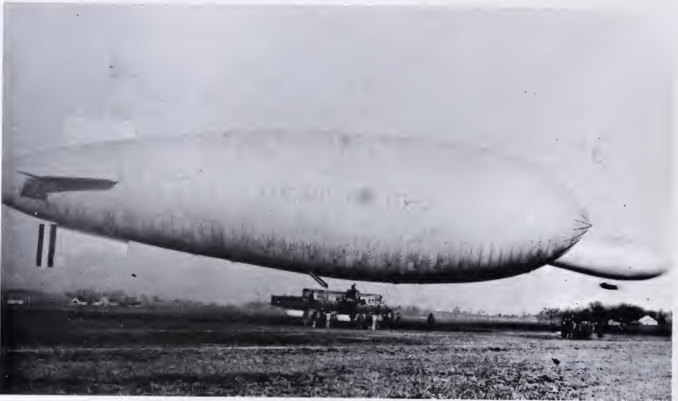
The 200,000 cubic foot TC-3 at Scott Field.
