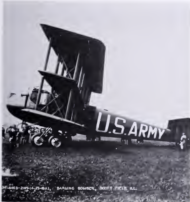
During the 1923 National Air Races in St. Louis, the Barling bomber, then the largest of its kind, visited Scott at least twice. This picture shows the Barling at the field on 14 September 1923. Weighing more than 42,000 pounds, the triplane could not get enough power from its six Liberty 12A engines to fly 100 mph or cross the Appalachians. The Barling did have a number of design features which proved useful in later aircraft. Despite its problems, the Barling impressed the public.
