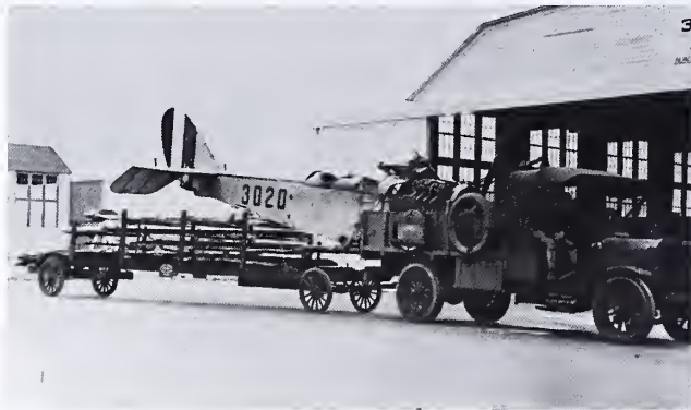
A wrecked plane on its way for repairs. Made of wood and cloth, planes would often be rebuilt several times.
