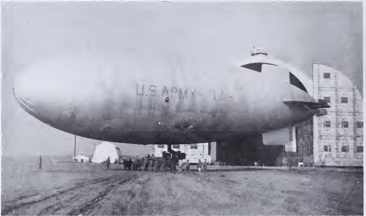
The non-rigid TA airship at the south end of the hangar. This training airship was a one-man control ship. The balloon and airship school used the TA as the next training craft after the free balloon.
