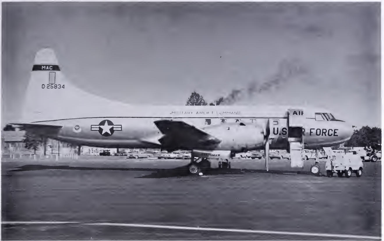
The Convair T-29—"a flying classroom," May 1967. The T-29 was the training version of the C-131A.
