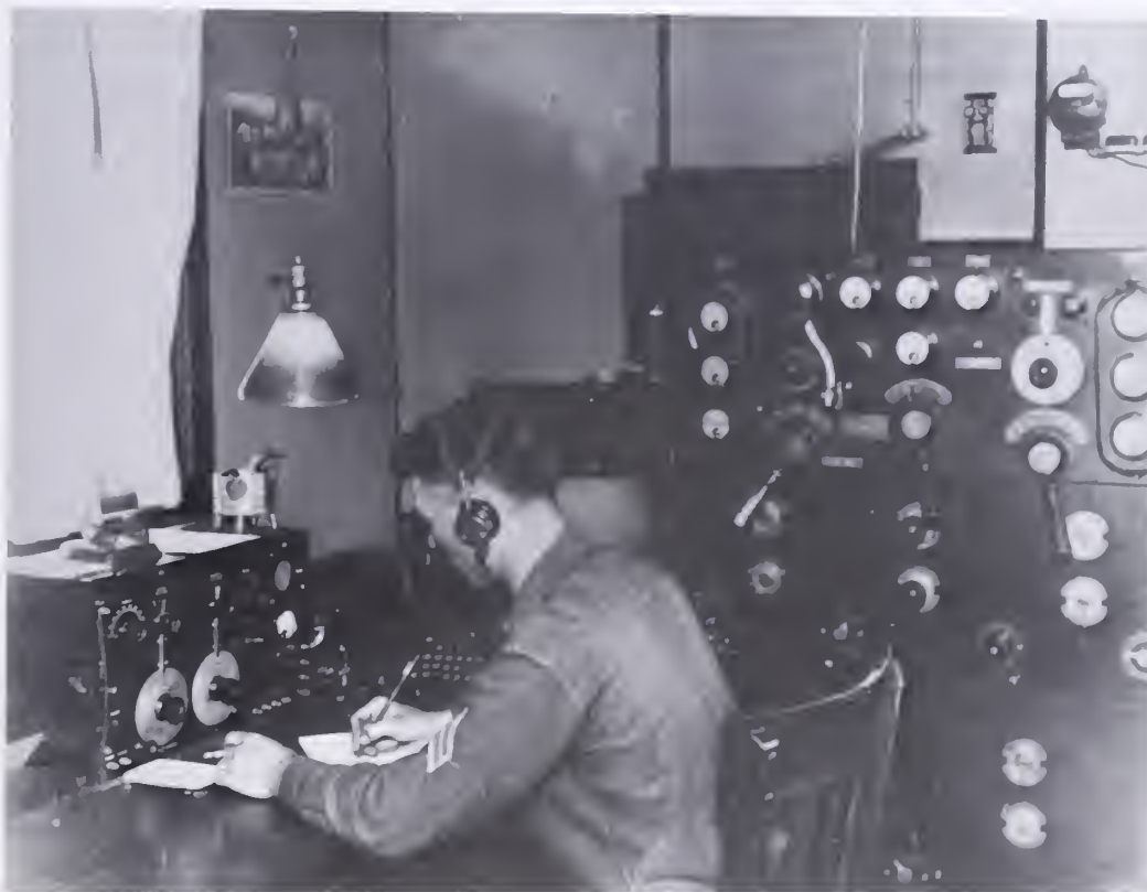
Scott's radio hut, June 1927. A detachment of the 6th Signal Service Company provided the field with communications—a life line welcomed by all balloon and airship pilots. The General Electric transceiver shown here had a range of 600 miles.
