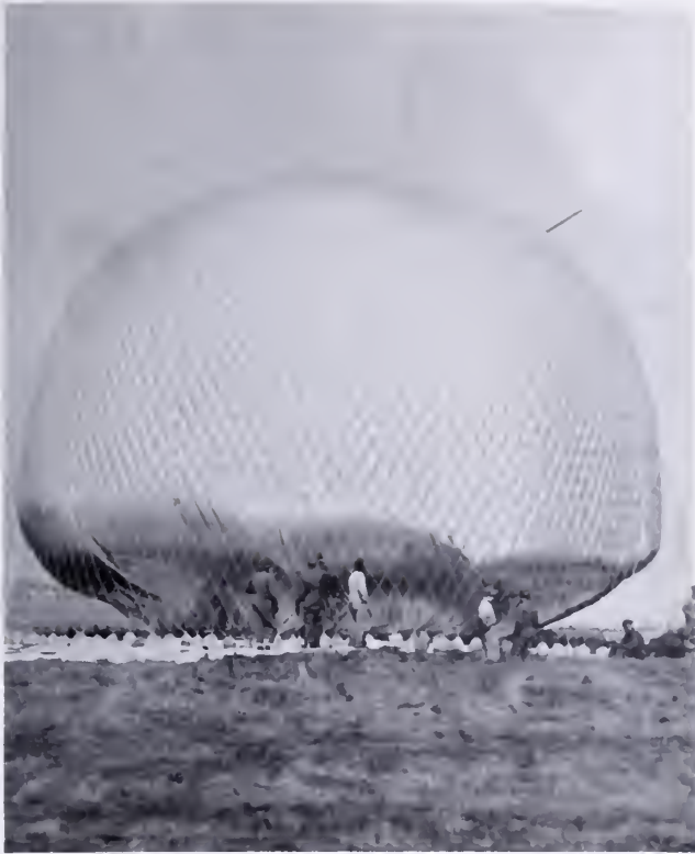
Inflating the 80,000 cubic foot free balloon for Captain Hawthorne C. Gray's world altitude record attempt, 9 March 1927. Gray used a rubberized and aluminum coated silk envelope with a silk net.
