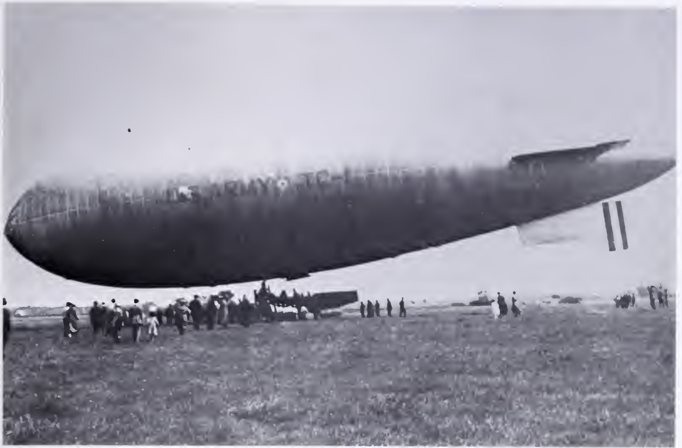
One of the few photographs of the TC-1, presumably at Scott Field. The $60,000 TC-1 was the first in a series of training airships which proved extremely durable. With a gas capacity of 206,000 cubic feet, it was, in its time, the largest non-rigid airship in the Air Service. It had an overall length of 195.8 feet and a diameter of 44.5 feet.
