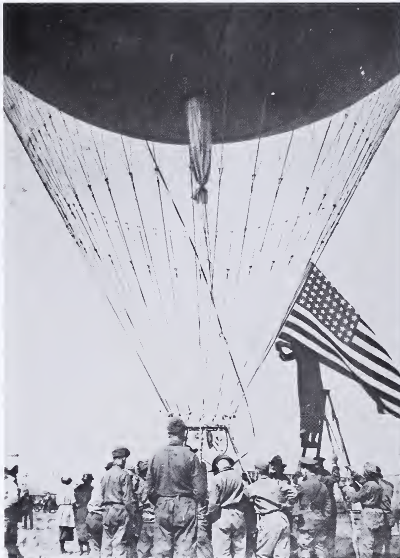
Final touches before the 35,000 cubic foot balloon cast off. Aboard for the first flight were Commander Chalmers Hall; Major Frank Kennedy; and Lieutenants Ashley McKinley, Angier Foster, and James Hill. The balloon also carried a wireless telephone.
