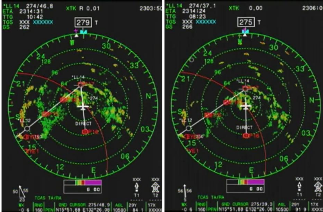
Figure 56. WC-130J aircraft radar imagery for TS Jangmi at (a) 2303 UTC 24 Sep, ~ 2 minutes before Dropsonde E splashed down at the ocean surface; and at (b) 2306 UTC 24 Sep, at the time of the splashdown of Dropsonde E. The exact location of the aircraft is shown with a white plane symbol. Dropsonde E is roughly located near the white aircraft symbol. The storm-relative position of Dropsonde E is shown in the plot at top center as in Figure 15a. There is only an area of weak convection near dropsonde in both radar images. The spacing between the range rings is 32 n mi. The following colors equate to the following radar reflectivity values: Green - > 25 dBZ; Yellow - > 35 dBZ; Red - > 45 dBZ; and Purple - > 55 dBZ.
