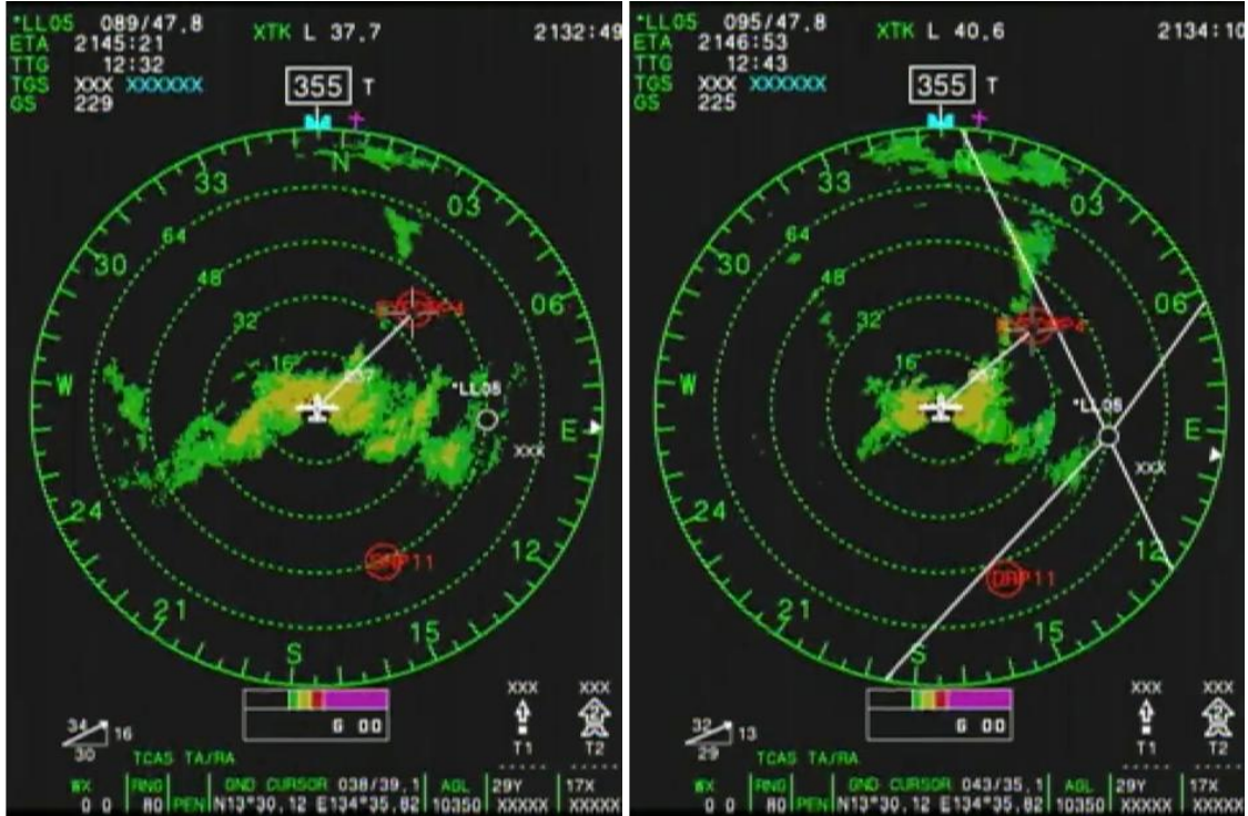
Figure 55. WC-130J aircraft radar imagery for TS Jangmi at (a) 2132 UTC 24 Sep, 2 minutes before Dropsonde D splashed down at the ocean surface; and at (b) 2134 UTC 24 Sep, at the time of the splashdown of Dropsonde D. The exact location of the aircraft is shown with a white plane symbol. Dropsonde D is roughly located near the white aircraft symbol. The storm-relative position of Dropsonde D is shown in the plot at top center as in Figure 15a. The dropsonde is located in an area of stratiform precipitation in both radar images. The spacing between the range rings is 16 n mi. The following colors equate to the following radar reflectivity values: Green - > 25 dBZ; Yellow - > 35 dBZ; Red - > 45 dBZ; and Purple - > 55 dBZ.
