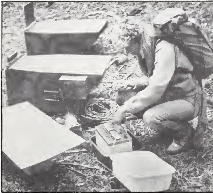
Enclosures used to measure filtered and unfiltered air as it passes over native seedlings in Giant Forest.
