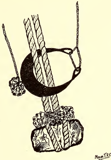
Fig. 7. The Datardu slipped around both the Heyers . The inner edge of the Datardu is sharpened like an ordinary sickle.
