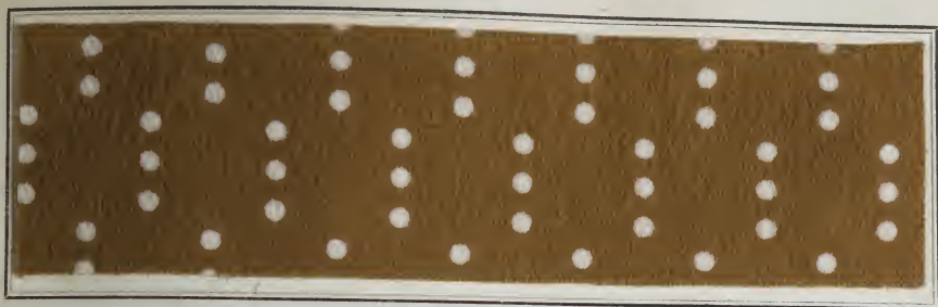
Padding Bath D. White Resist I , aged 5 min. Mather-Platt steamed \frac{3}{4} hour with \frac{1}{4} atmosphere pressure.
