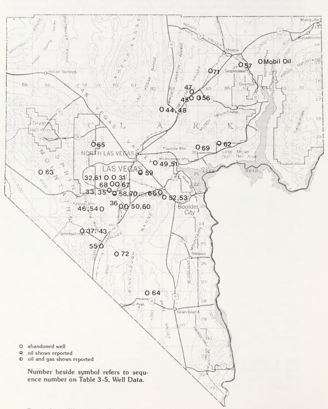
Figure 3-7. Wells drilled for oil and gas in Clark County, Nevada through 1979. (Modified from Garside and Shilling, 1977.)
