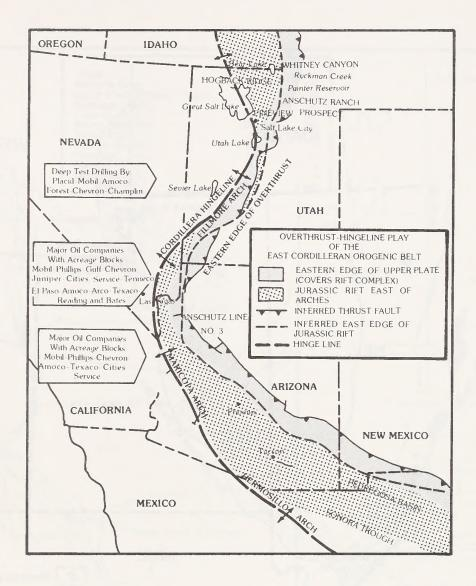
FIGURE 3-4. Interpretation of where the Overthrust Belt and Cordillera Hingeline occur in Arizona and Nevada from the Anschutz Corp. (Oil and Gas Journal, July, 1979)
