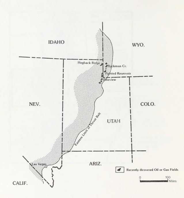
Figure 3-5. Interpretation by Chevron, Inc. (1979) of where the Overthrust Belt occurs in Nevada and Utah. Western Limit is not defined.
