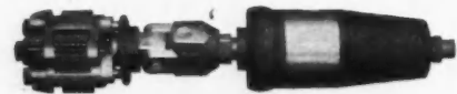
Fig. 2 Rotary type of cleaner for curved tube boilers such as the Badenhausen or Sterling boilers. Not usable on fire tube boilers.
