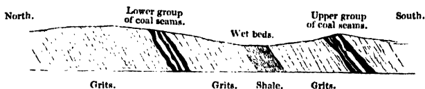
Fig. 1.—Section across the coal-field of Ancenis.
