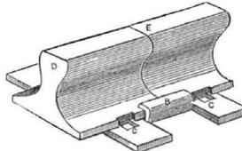
the rail secured in the chair, and figure 2 is a perspective view of the chair itself. D E are the sections of two rails placed together and secured at the joint on the chair by the jaws,
