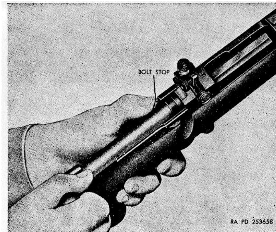
Figure 28. Removing bolt from receiver (Winchester rifle model 70).
