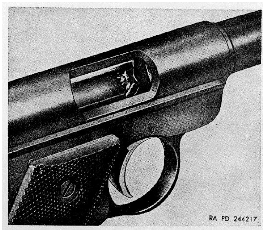
Figure 36. Inspecting chamber after unloading pistol (Ruger).
