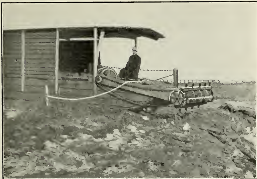
FIG. 1.—POWER-DRIVEN MACHINE FOR FREEING CHANNELS OF SEDGES AND SALT GRASSES, MISSEGUASH MARSH, NEW BRUNSWICK.
