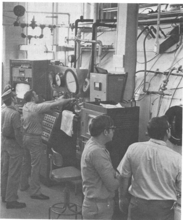
MONITORING AIR-SATURATION DIVE. —The 30-day confinement period began on 1 Oct 1973, in the cylindrical chamber used originally in the Sealab Project. One of the Navy's most comfortable models, the chamber measures 9 ft in diameter. Watching pre-decompression activity closely (from left to right) are: BMCM Michael Oranczak (obscured from view); TM2 Gary Seibert; HMCS Jack Caldwell; LCDR G.M. Adams, MSC, USN; and ENC James Jordan, USN (Ret.).
