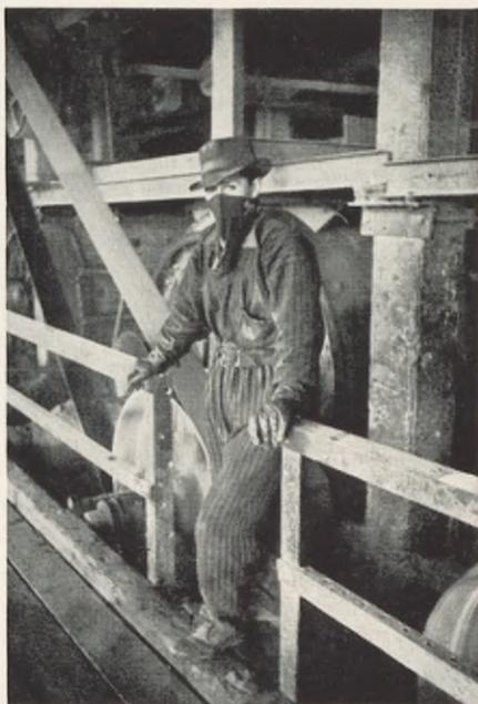
*Handkerchief used as a protection against acid mist in a copper smelter*
