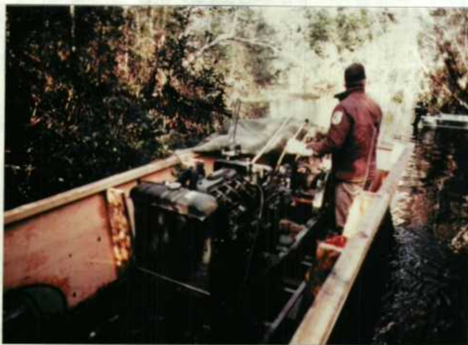
This "homemade" log puller was constructed by refuge personnel using excess materials and was very effective in removing logs from the canal. 83-13-JAB (03/83)
