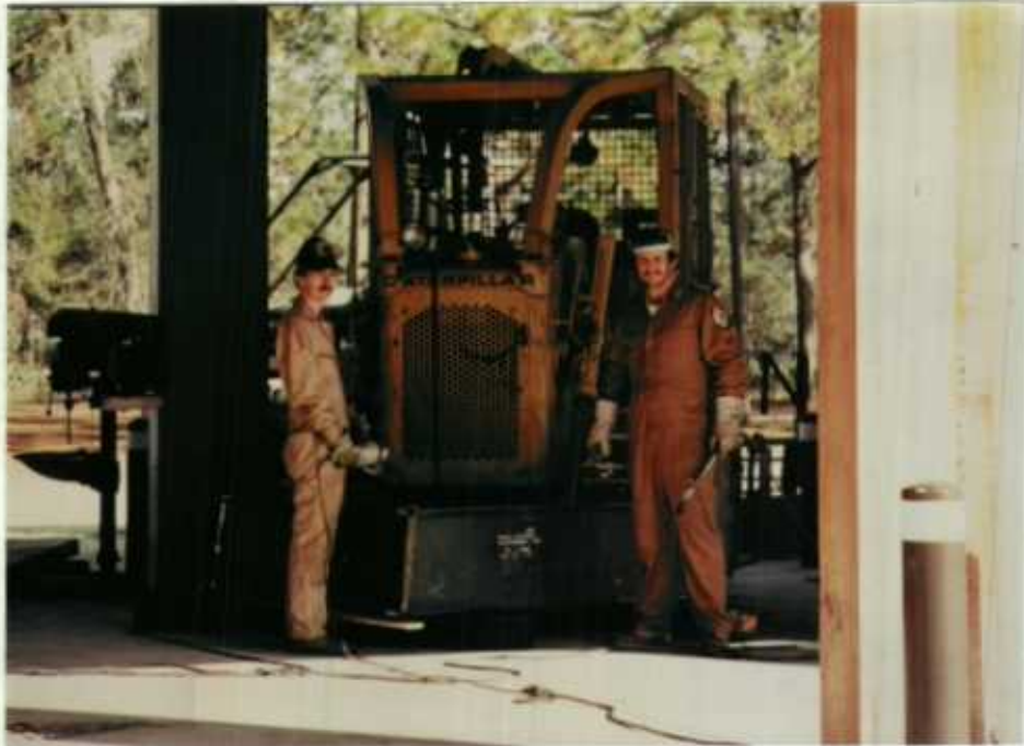
Biological Technicians Doug Nuss (right) and Tony Gooch designed and fabricated this V-blade from excess material for the D-4 dozer. 83-15-WCK (01/83)
