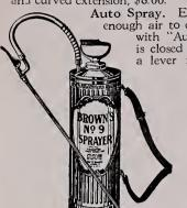
Auto Spray. Eight to ten strokes, compresses enough air to discharge entire contents. Fitted with "Auto Pop" automatic valve, which is closed by the air pressure. In operation a lever is moved, opening the valve and
