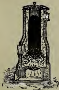
Base-Burning Water Heaters for Small Greenhouses, Con- servatories, Etc.
