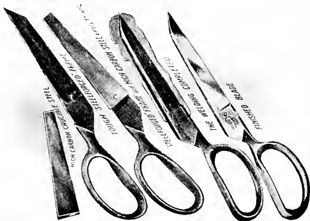
Figure 6. From Bar of Steel to Finished Blade
