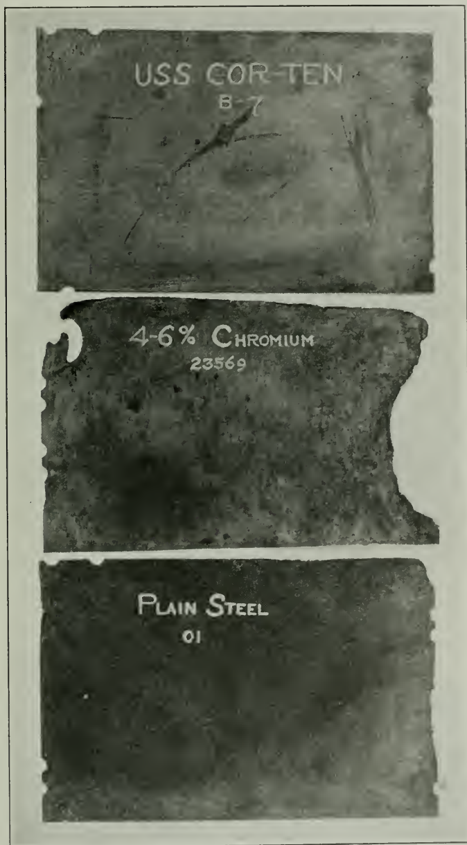
FIGURE 5.—USS COR-TEN is more durable in running mine water of an acid nature than other steels. These samples were immersed for eight weeks.
