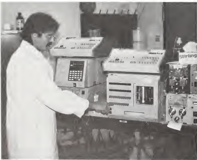
High performance liquid chromatography is used to determine the presence of specific residues in meat and poultry products.
