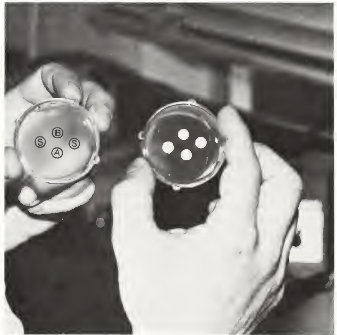
The species identification field test, SIFT, was developed to detect product adulteration which will aid in the elimination of economic fraud.
