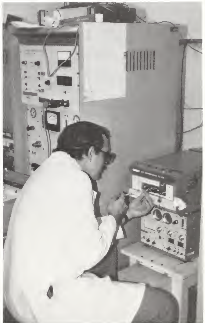
Thermal Energy Analyzers are used to determine the nitrosamine content in samples of cured pork product.
