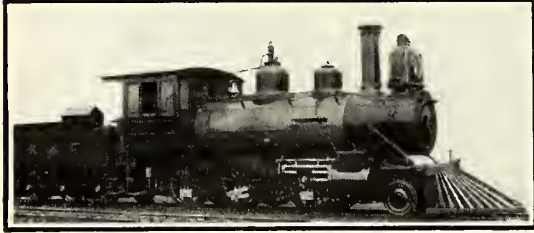
A MOGUL TYPE FREIGHT-LOCOMOTIVE OF 1890.
