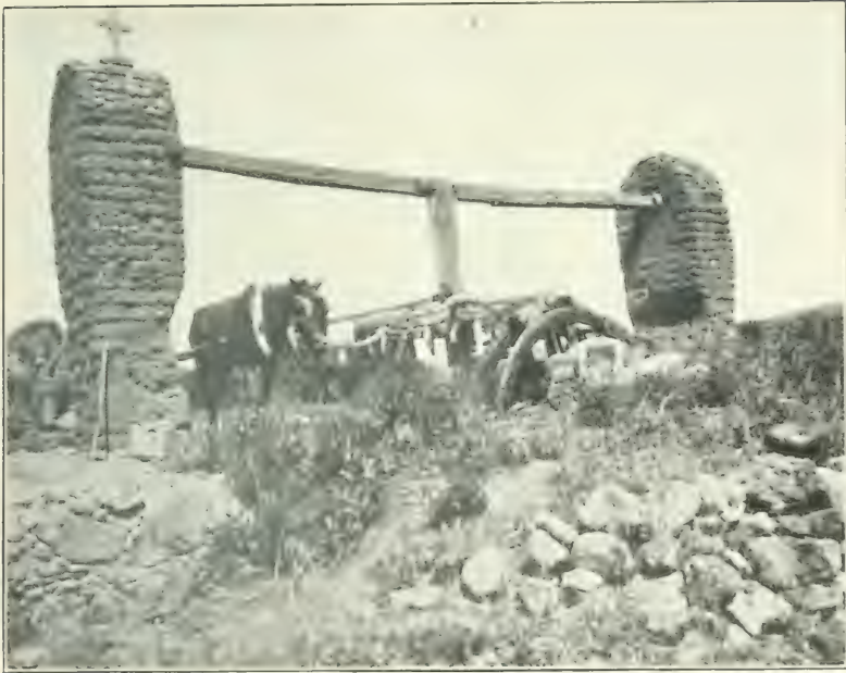
A PRIMITIVE CONTRIVANCE FOR RAISING WATER FOR IRRIGATION. The horse turns a large horizontal wheel. The vertical pegs on the under side engage a similar series on the side of the vertical wheel, which in turning raises a line of buckets on the circumference. The supporting pillars are of adobe. Near Zacatecas.
