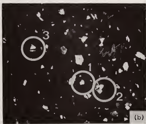
Figure 2. Identification of grains of 304 stainless steel. (a) Metallograph. (b) X-Ray reflection micrograph. Crystal-monochromated \text{CrK}_{\alpha_1} radiation.
