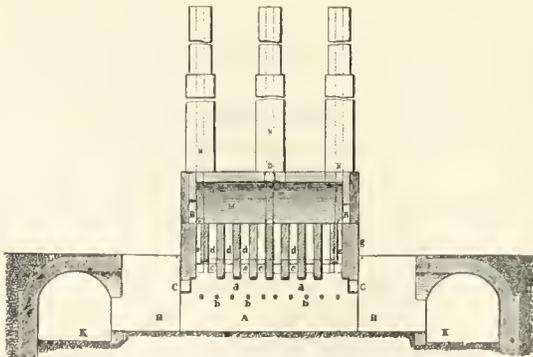
FIG. 6.—Cementing furnace (vertical section).
