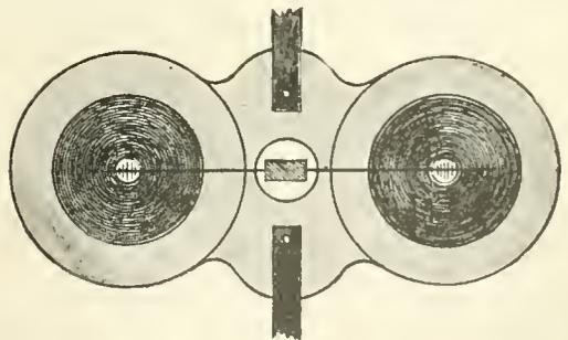
FIG. 8.—Needles, mirror, and rear coils of a sensitive astatic galvanometer.
