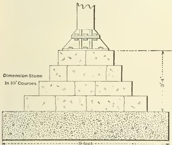
FIG. 12.—Masonry footings in concrete.
