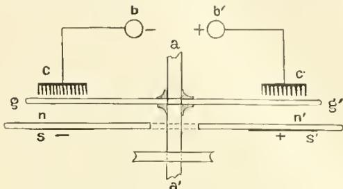
Fig. 4.—The essential parts of the Holtz machine.
