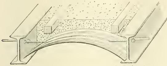
FIG. 3.—Concrete fillings on corrugated-metal arches.
