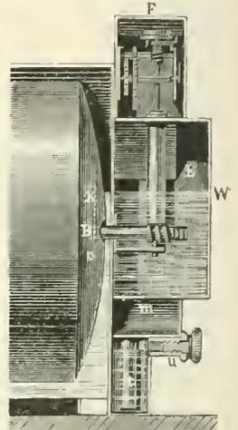
FIG. 3.—Section of the modern wet meter, shown also in Figs. 2 and 4, described under Fig. 2.
