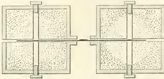
FIG. 9.—Cross-section of coils of a sensitive astatic galvanometer.
