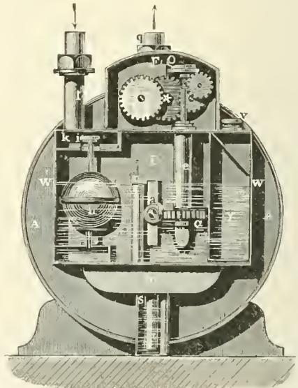
FIG. 4.—Front section of the modern wet meter, shown also in Figs. 2 and 3. *a* is the screw on the axis of the drum which turns the toothed wheel *a*, the axis of which passes through the tube *e* to the system of wheels in the space *F* which move the hands on the index-dials shown in Fig. 7.
