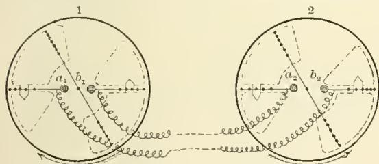
FIG. 4.—The Holtz machine driven as a motor.
