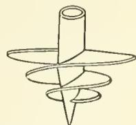
FIG. 8.—Screw pile.
