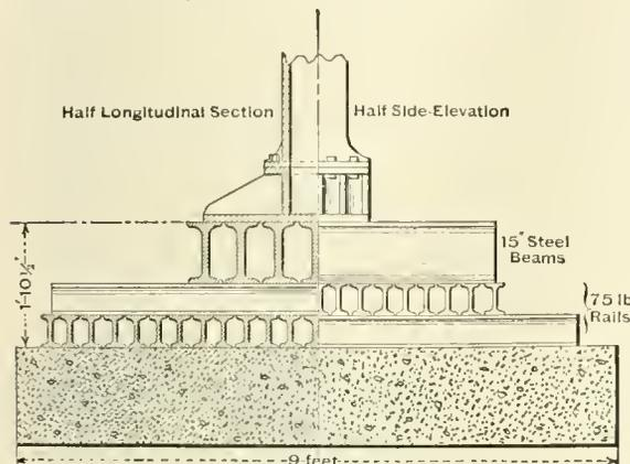
FIG. 11.—Iron-rail footings in concrete.
