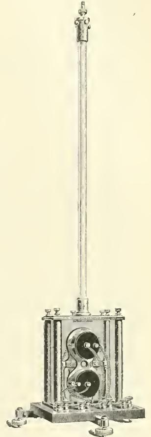
FIG. 7.—A sensitive astatic galvanometer with four coils.
