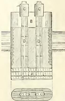
FIG. 21.—Pneumatic pier.
