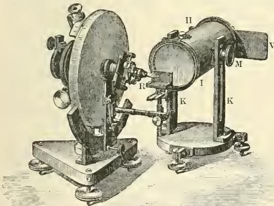
FIG. 5.—Wollaston's goniometer and Mallard's collimator.
