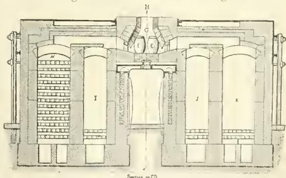
FIG. 16.—Siemens gas-pot furnace (cross section).
