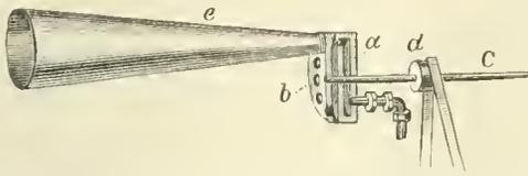
*Explanation.*—*a*, Steam drum, with one hole on front face; *b*, revolving plate, perforated with eight holes and supported on the shaft *c*; *d*, a pulley, to which rapid motion is given by a band and driving-wheel; *e*, resonator or trumpet.
