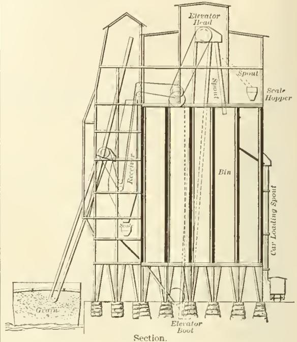
which are laid on and fastened to the supporting columns, and the bins vary in height from 60 to 80 feet, and are from 10 to 12 feet square. The floor of the building on top of
