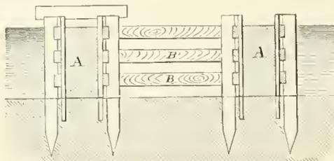
FIG. 14.—Coffer-dam, showing detail.
