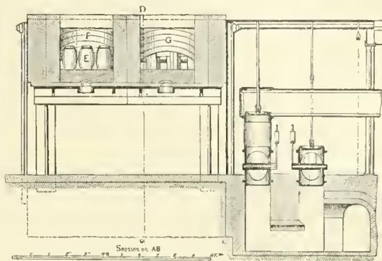
FIG. 15.—Siemens gas-pot furnace (longitudinal section).
