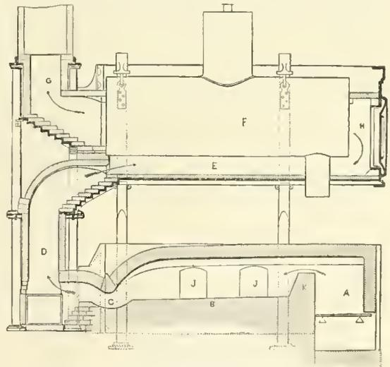
FIG. 3.—Reverberatory heating furnace (vertical section).
