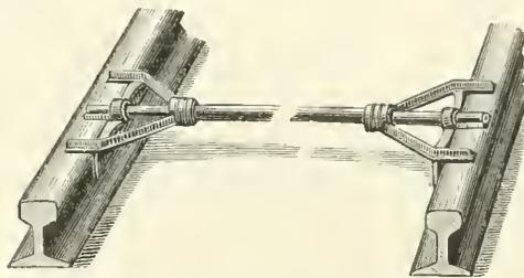
tance apart. On curves the gauge of the track is often made slightly wider than on the straight portions, and hence the ends of the implement are adjustable, and they are sometimes made with segments of a circle corresponding in curvature to that required for the rails. See RAILWAYS concerning the narrow gauge, standard gauge, and broad gauge. MANSFIELD MERRIMAN.
