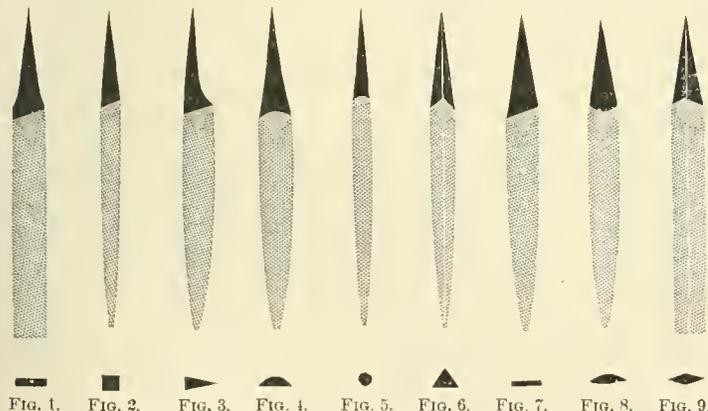
hibits the half-round file, the section of which, as seen, is not a complete semicircle. The thickness of the file is usually from one-half to one-fourth the radius of the circle. Fig. 5 represents the round file. If of small size it is called, when tapering, a rat-tail file, and when parallel a joint file or gulleting saw file. Fig. 6 represents the triangular file, often called by the workman a three-square file. It is used for sharpening saws, for cutting internal angles,
