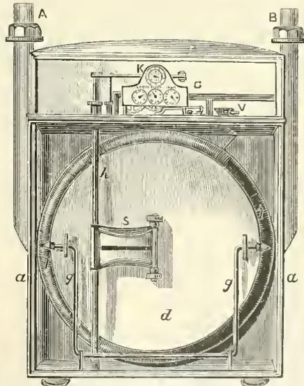
FIG. 6.—Front view of the dry meter. A is the inlet, B the outlet. The gas enters at A, passes to the valve-box V, enters the space 2 (Fig. 5), and the left-hand chamber *l r*, while its pressure forces the gas out of the space 3 and the right-hand chamber *r l*. When the left-hand chamber is full and its companion empty, the slide-valves reverse the flow of gas, and the empty chamber and the space 3 receive, while the full chamber and the space 2 deliver gas.
