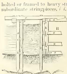
FIG. 13.—Section of coffer-dam: *a*, main exterior piles; *b*, strong square beams, corresponding to *a*, on which the wales *u u* are notched and bolted; *c*, sheeting-piles; *e*, cross-pieces; *o o*, horizontal shores buttressing opposite sides of dam; *A*, puddling; *B*, interior space; *C*, mud, etc.
