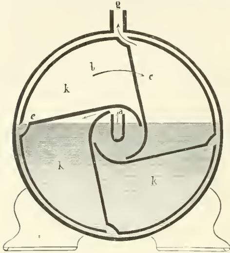
FIG. 1.—Vertical section of the early wet meter. The gas enters the chambers *k* at the center through the tube *a*, and passes out through the slits *e* on the periphery of the drum, escaping at the outlet *g*.
