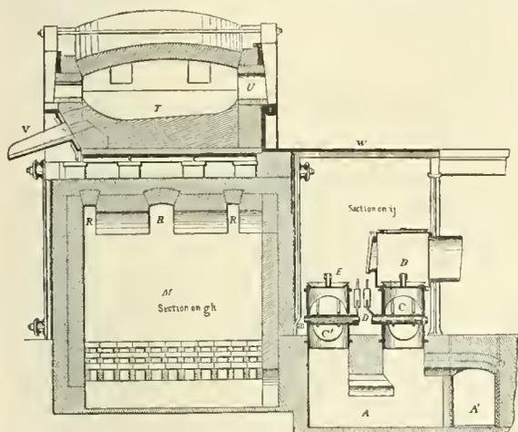
FIG. 13.—Siemens gas-furnace (cross-section).
