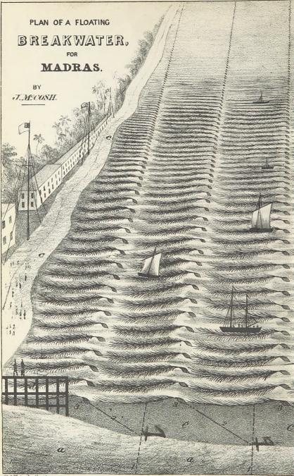
RR.Roadstead. a.Sandy Bottom. C.Vertical Section of water: c. Strand, d.Wharf. 1. Cables & Anchors. 3. Lines of Baoys. 2. Baoy Ries. 4. Trucking Baoys: & Ropus CHARMAN THAT a a
