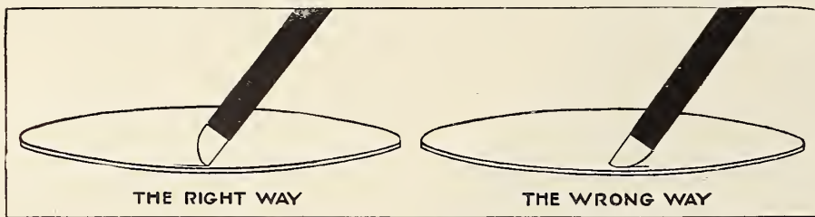
HOW TO ADJUST PERMANENT JEWEL NEEDLE.
