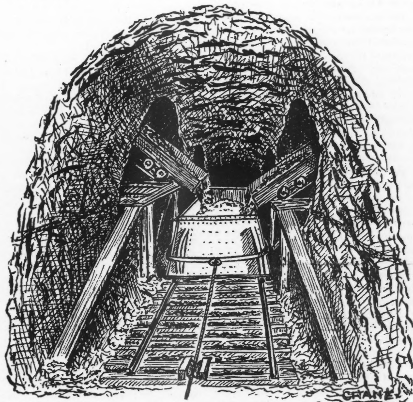
FIG. 5. PIT-CAR DUMPING INTO SKIP.
