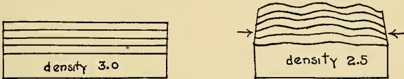
FIG. 1.—Diagrams showing the decrease in density in depth below a mountain range due to the reducing of the overburden by support from the sides and the formation of lava in place.
