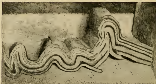
FIG. 7.—Same model as Fig. 6, compressed to total of 8 inches. Cavity has disappeared with more intense folding. Other tiny cavities have developed where the folding is gentle. The overturned fold of Fig. 6 has become nearly upright.
