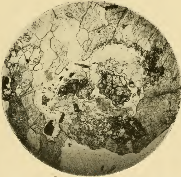
FIG. 3.—Garnet in limestone. (Magnification about 30 diameters. Ordinary light.) The photograph shows garnet (high relief) in the center of the field; it is surrounded by a broad kelyphite rim, which seems to be an incipient stage in its formation. The remainder of the field is largely carbonates.
