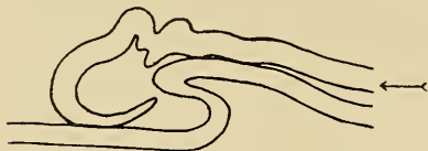
FIG. 15.—Broken overturned fold. The front of the fold has turned under, resembling the so-called head of a nappe. Two nappes in different stages of development formed by compressing a single layer of equal parts of paraffin and vaseline.
