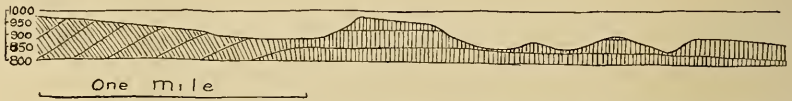
FIG. 6.—Longitudinal profile of the deepest of the Drumheller Channels across the nose of the anticline. Four rock basins are indicated, the largest of which is 75 feet deep.
