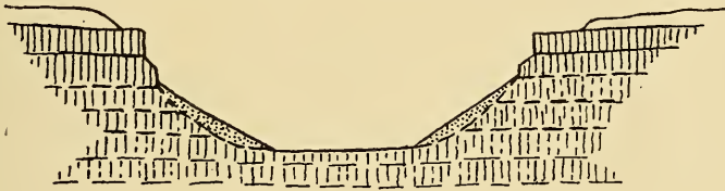
FIG. 10.—Devils Canyon, cross-section a mile and a half south of Kahlotus, showing (1) steepened loessial bluffs ( 33^\circ ), (2) narrow scabland above brink of basalt cliffs (3) canyon 450 feet deep and less than one-fourth mile wide, and (4) post-Spokane talus, three-fourths the height of the cliffs. Horizontal and vertical scale the same.
