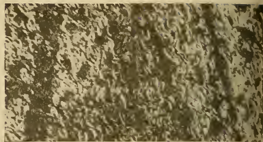
FIG. 8.—Section ( \times 118 ) crosswise to the bedding of coal from the Primrose bed, William Penn colliery. This section through the duller layers shows wood fiber much contorted.
