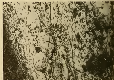
FIG. 10.—Section ( \times 124 ) crosswise to the bedding, from Pennsylvania Anthracite. This section through the duller layers shows a somewhat macerated wood fragment containing round bodies which are probably vessels formerly filled with resin or gum.
