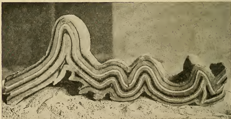
FIG. 8.—Reverse face of Fig. 7 model. Pressure from the left. Vertical variations of folds.
