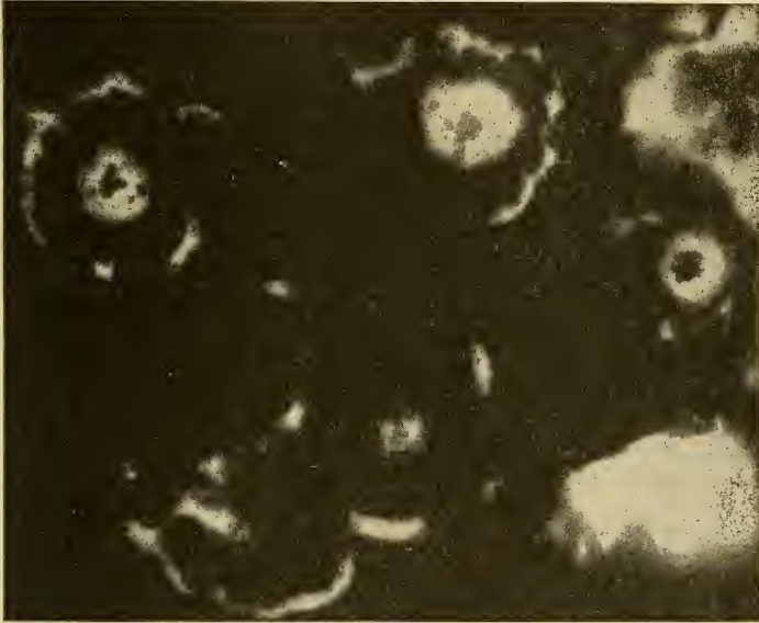
FIG. 4.—From same thin section as Figures 2 and 3. Show segregation of iron oxide into hematite plates and also original banding outside the area of segregation. Magnified 430 diameters.
