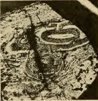
FIG. 2.—Section ( \times 170 ) crosswise to the bedding, from Pennsylvania anthracite. Shows large, wrinkled spore exines found in the duller layers.
