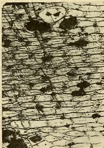
FIG. 5.—Section ( \times 126 ) crosswise to the bedding and oblique to an apparent stem in anthracite from Pennsylvania. This section is of particular interest because it is in the brilliant jetty coal and not in the duller layers where such forms are usually found.
