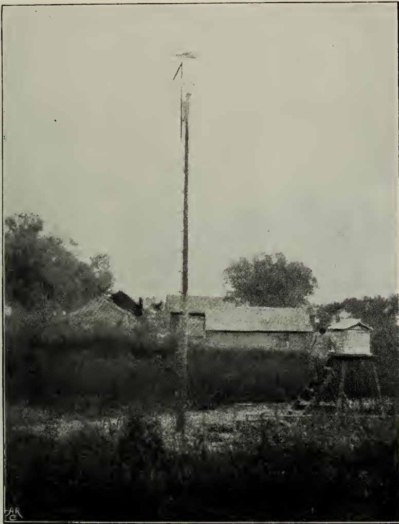
Instruments for meteorological observations erected in village of Ching-yun-p'u, summer of 1905, at the head of the line of communication of the 2nd Army. The pole for the anemometer was made and used at Liao-yang, and had been carried about from place to place as the army advanced.
