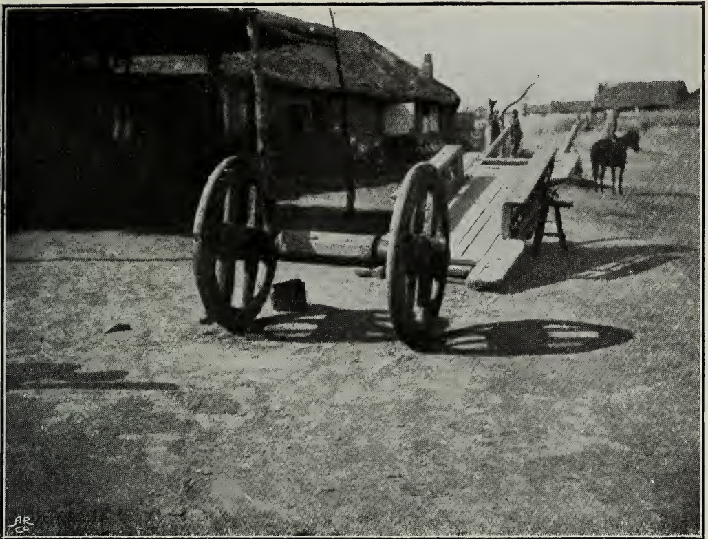
Same cart as 7 and 8, showing detachment of wheels from body.
