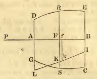
Let P be a body situated in the axis A B of the curve D E C G, by the revolution of which the solid is generated. Let any circle R F S perpendicular to the axis, cut the solid, and in the semidiameter F S of the solid, take F K proportional to the attraction of the circle on P, then F K. F f  $\alpha$  attraction of the solid whose base = circle R F S, and depth = F f, let I K L be the curve traced out by F K,  $\therefore$  A L K F  $\alpha$  attraction of the solid.
