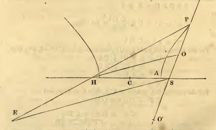
V<sup>2</sup> down O P : V<sup>2</sup> in the circle rad. S P :: O P :  $\frac{S O}{2}$ V<sup>2</sup> in the circle S P : V<sup>2</sup> in the hyperbola at P :: A C : H P
