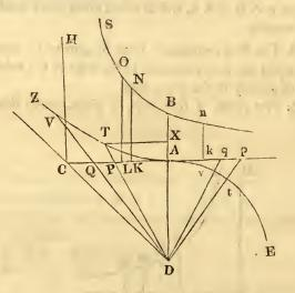
pendicular and equal to it. With the center D and radius A D describe the quadrant A t E and the hyperbola A V Z. Draw the radii D P, D p. Then
