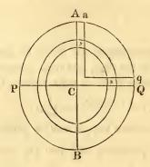
the pole : force of gravity at the equator :: 289 : 288. Suppose A B Q q a spheroid revolving, the lesser diameter P Q, and A C Q q c a a canal filled with water. Then the weight of the arm Q q c C : ditto of A a c C :: 288 : 289. The centrifugal force at the equator, therefore 1 suppose  $\frac{1}{289}$  of the weight.
