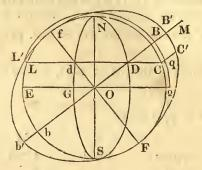
As the point D is carried along its parallel of latitude, it will pass through all the states of the tide, having high water at C and L, and low water when it comes to (d) the intersection of its parallel of latitude with the equator of the watery spheroid.
