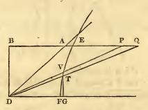
$\alpha A B^2 - B D^2$ . Draw D F parallel to P B and = D B and with the center D  $-\frac{1}{2}$  axis-major =  $\frac{1}{2}$  axis-minor = D B, describe a hyperbola from the vertex F, cutting A D produced in E, and D P, D Q in T, V.
