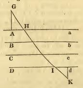
Take A H = I d, and draw A G, d K perpendicular upon A a, D d, meeting the directions of incidence and emergence in G, K. Let the motion of the body be resolved into the two G A, A H, I d, d k, the ve-
