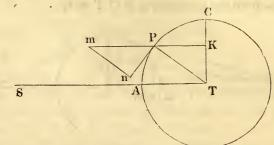
If P T equal the addititious force, then the ablatitious force equals 3 P K, for P K : P T : : sin.  $\theta$  : (1 = r),
