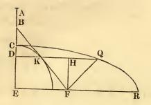
Let A C and E be the respective places of the object, eye, and reflector at first, and B Q and F their places at any other time, or if K F = F Q = C E, K may also be the place of the eye, and since K F always = C E, and that B F is constant, K will trace out an ellipse by next problem. Also by optics the angle K F H = H F Q, and from similar triangles,
