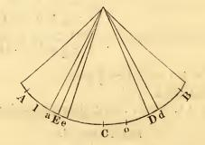
non-resisting medium in any time. Then the accelerating force at any point  $D \propto C D$ ; let C D represent it, and since the resistance  $\infty$  time, it may be represented by the arc C o.
