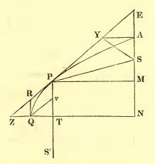
Let u be the velocity resolved parallel to P M then since the force acts perpendicular to P M, u at any point must be same as at A,  $\therefore$  if P Q be the velocity in the curve, QT = u = constant quantity, and  $a = \frac{S' P \cdot Q T}{2}$  $\frac{S' P \cdot u}{2}$ .
