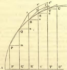
Let P P' = y be any fixed or definite ordinate of the curve A U, and taking P' Q' = Q' R' = R' S' = &c. let ordinates be erected meeting the curve in Q, R, S, T, &c. Join P Q, Q R, R S, &c. and produce them to meet the ordinates produced in r, s, t, &c. Also draw r s', s t',
