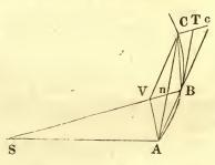
generated by the incessant force in the time through A B, is C c. But if the force had been incessant instead of impulsive, the body would have been moving in the tangent B T at B, and in this case the deflection at the end of the time through B C would have been half the space described with the whole velocity generated through B C (Wood's Mech.) But
