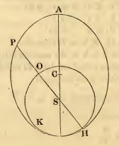
Time of fall = time of describing  $\frac{\text{circle}}{2}$  O K H, S O =  $\frac{\text{S P}}{2}$ ,  $\frac{\text{period in the circle O K H}}{\text{period in the ellipse}} = \frac{\text{period in the circle rad. S O}}{\text{period in the circle rad. A C}} = \frac{\text{S O}^{\frac{3}{2}}}{\text{A C}^{\frac{3}{2}}}$
