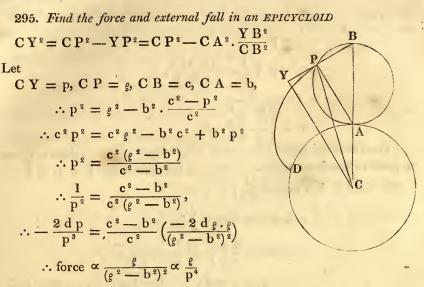
(as in the Involute of the circle which is an Epicycloid, when the radius of the rota becomes infinite.)
