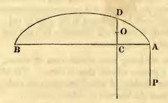
Let w = weight of the string. L = length. D d : L : : weight D d : w  $\therefore$  weight of D d =  $\frac{D d \times w}{L}$
