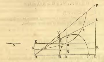
let D A : A C :: resistance : gravity. Also D P : C P :: resistance : gravity,  $\therefore D A \times D P : C P \times C A :: R : G$ . Between D C, C P describe a hyperbola cutting D G and A B perpendicular to D C in G and B, from R draw R V perpendicular cutting D P in V and the hyperbola in T, complete the parallelogram G K C D and make N : Q B :: C D : C P.
