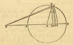
Draw E D, e d perpendiculars upon P S; let e d intersect E F in r; draw r n perpendicular upon E D. Then E r: n r:: P E: E D,  $\therefore$ E r. E D = n r. P S = D d. P E,  $\therefore$  the annular surface generated by the revolution of E r  $\alpha$  E r. E D  $\alpha$  D d. P E, and (P E remaining the same)  $\alpha$  D d. But the attraction of this annular surface on P  $\alpha$  D d. P E, and the attraction in the direction P E: the attraction in the direction P S:: P E: P D,
