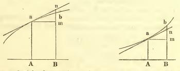
Let y = f(x) be the equation to the curve a b; then A a, B b being any two ordinates, and a n a tangent at the point a, if we put A a = y, and A B = h, we get
