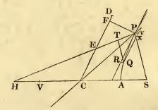
175. If the centripetal be changed into a repelling force, and the body revolve in the opposite hyperbola,  $F \propto \frac{1}{H P^2}$ .
