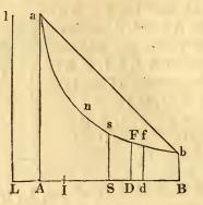
Take S I=S s, and describe a hyperbola passing through a, s, b, to which L l, L B are asymptotes; then as in the former case, the area A a n b B = A L.S B.  $\int \frac{L B}{L A} = L S. S s \int \frac{L B}{L A} = S I.L S \int \frac{L B}{L A}$  $\therefore$  the area A N B = S I.L S  $\int \frac{L B}{L A} - S I.A B.$
