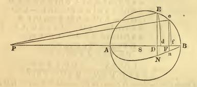
For the attraction of lamina E F f e  $\alpha$  D E<sup>2</sup>. F f × force of each particle  $\alpha$  (LEMMA XXIII)  $\frac{D E^2 \cdot P S}{P E}$ . D d × force of each particle, or  $\alpha \frac{D E^2 \cdot P S}{P E \cdot V}$  D d,  $\therefore$  D N · D d  $\alpha$  attraction of lamina E F f e, and the sum of these areas or area A N B will represent the whole attraction of the sphere on P.
