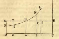
Describe the hyperbola G B K between the asymptotes A C and C H cutting the perpendiculars D E, d e, in G and g.
