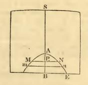
... the quantity effluent through the whole area A m S t A = sum of all the portions effluent through M N =  $\int 2 y x' \sqrt{g h' + x t} - 2 t$  $\sqrt{g f} \sqrt{h' + x} + C$  connected between the values x = 0, and x = h - h'.
