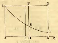
The space described in the time A H with the first velocity continued uniform : space described in the resisting medium, in the same time : : A H P L : area A L S H : : rect. A L  $\times$  P L : rect. A L  $\times$  P S\* : : P L : P S (if A L = subtan. of the curve).
