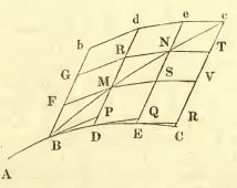
Let a body move in the curve A B C, and when at B, let an additional force act upon it in the direction B b. Also let B D, D E, E C; B F, F G, G b be spaces that would be described in equal times by the body moving in the curve, and when moved by the sole action of the new force. Then draw tangents at the points B, D, E meeting D d, E e, C c, each parallel to B b, in P, Q, R. Also draw F M, G R, b d parallel to B P; M S, R N, d e parallel to D Q; and S V, N T, c c parallel to E R.
