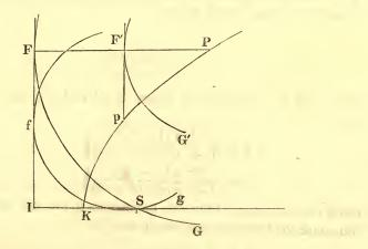
But this is done by describing from P with a radius = S P - S p, a circle F' G', by drawing from p the tangent p F' as in the other case (or by describing a semicircle upon P p, so as to intersect F' G' in F') by producing P F' to F, and drawing F f parallel to F' p.
