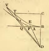
With center D and vertex B, describe the rectangular hyperbola B T V, cutting the lines D A, D P, D Q produced in E, T, V.
