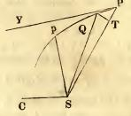
d. area =  $\frac{\varrho^2 d \theta}{2}$ ,  $(\theta = \angle C S P)$ , for d. area =  $\frac{Q T \cdot S P}{2}$ .
