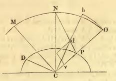
The velocity-curve is a straight line, (since D F  $\alpha$  C D, also since F = 0, when C P = 0, this straight line comes to C, as C d b, V  $\alpha \sqrt{COb} \alpha$  C O, O being the point fallen from, to acquire V at P.
