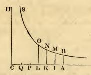
15. PROP. VIII. Let C A represent the force of gravity, A K the resistance,  $\therefore$  C K represents the absolute force at any time (if the body descend); A P, a mean proportional to A C and A K, représents the velocity; K L, P Q are contemporaneous increments of the resistance and the velocity.
