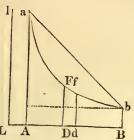
∴ area A a F D =  $\int D F \cdot D d = A L \cdot L B \int L D$ , ∴ hyperbolic area A a f b B = A L · L B  $\int \frac{L B}{L A}$ .
