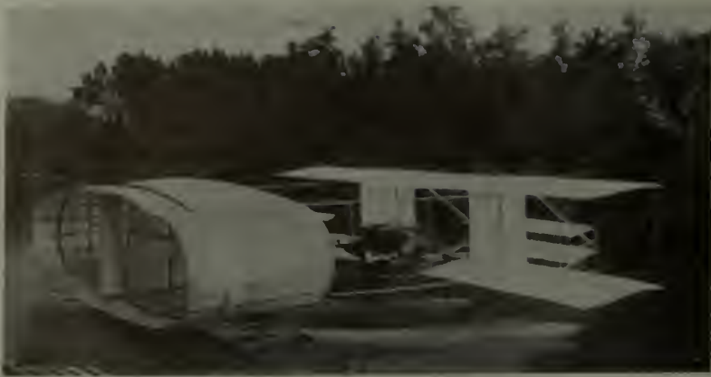
A French hydro-aeroplane that is being used for experimental purposes. It is a biplane with a barrel tail, mounted on a catamaran
