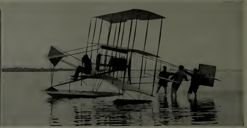
A triplane of great lifting power which Curtiss used in his experiments but discarded. Note the central float and the buoys at the sides
