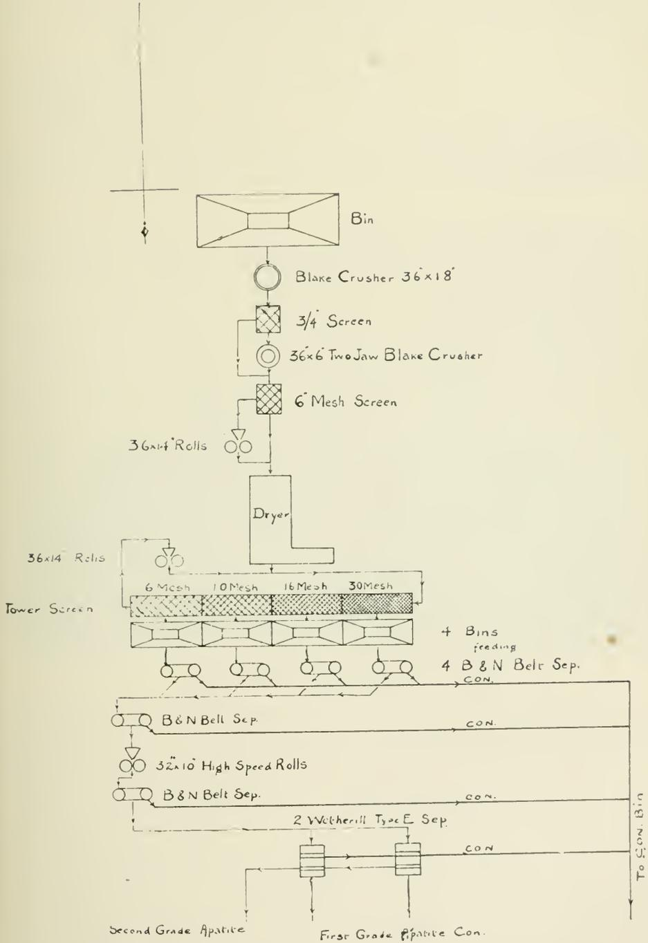
Flow sheet of No. 2 mill ; Witherbee Sherman & Company, Mineville, N. Y.
