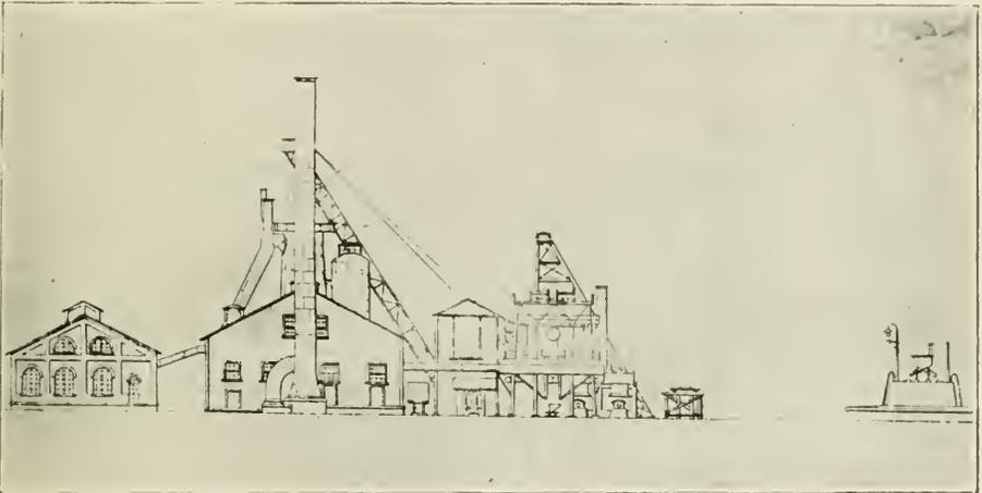
Atikokan Iron Company. Elevation east end of plant, showing power house, boiler house, skip hoists, roaster and bee hive coke ovens.
