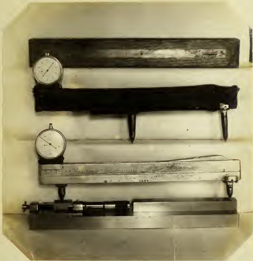
Fig. 16. Standard Bar, Extensometers and Calibrating Device.
