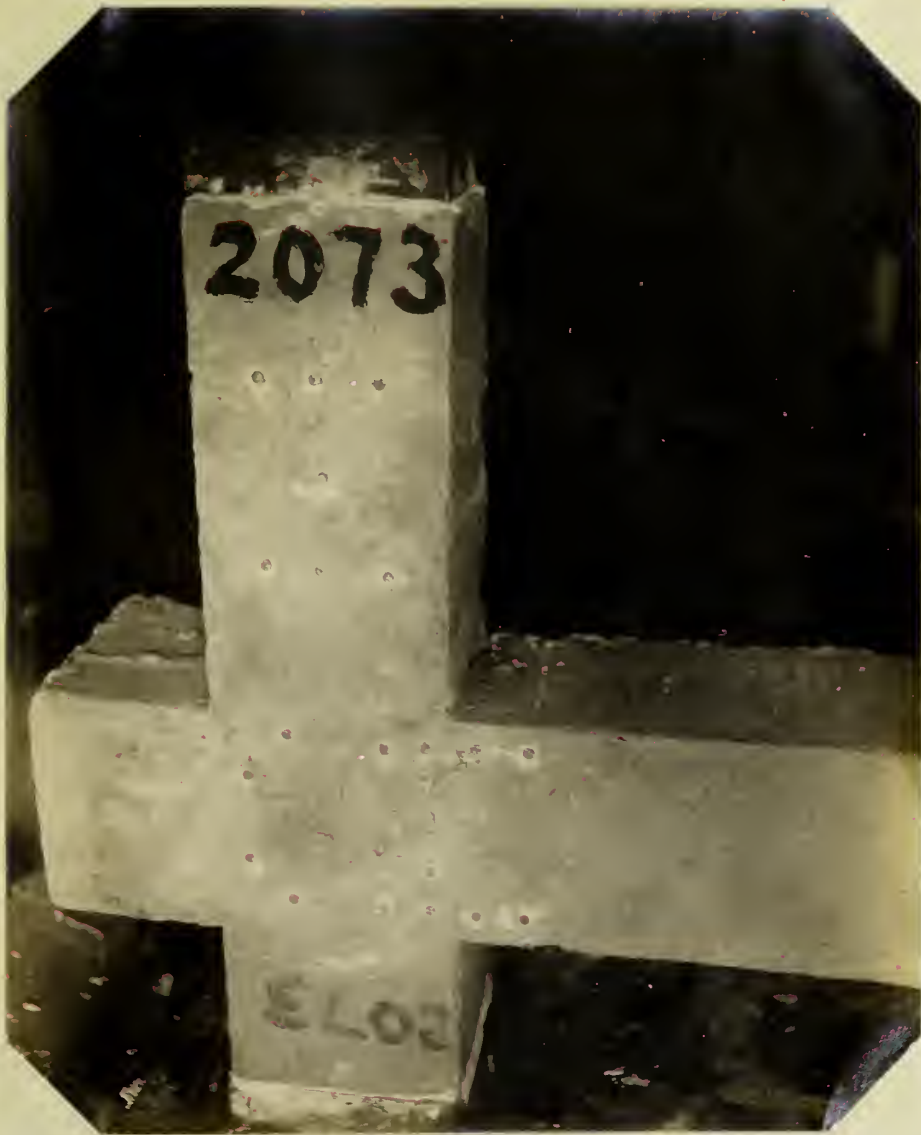
Fig. 24. Compression Specimen 2073 at Failure.
