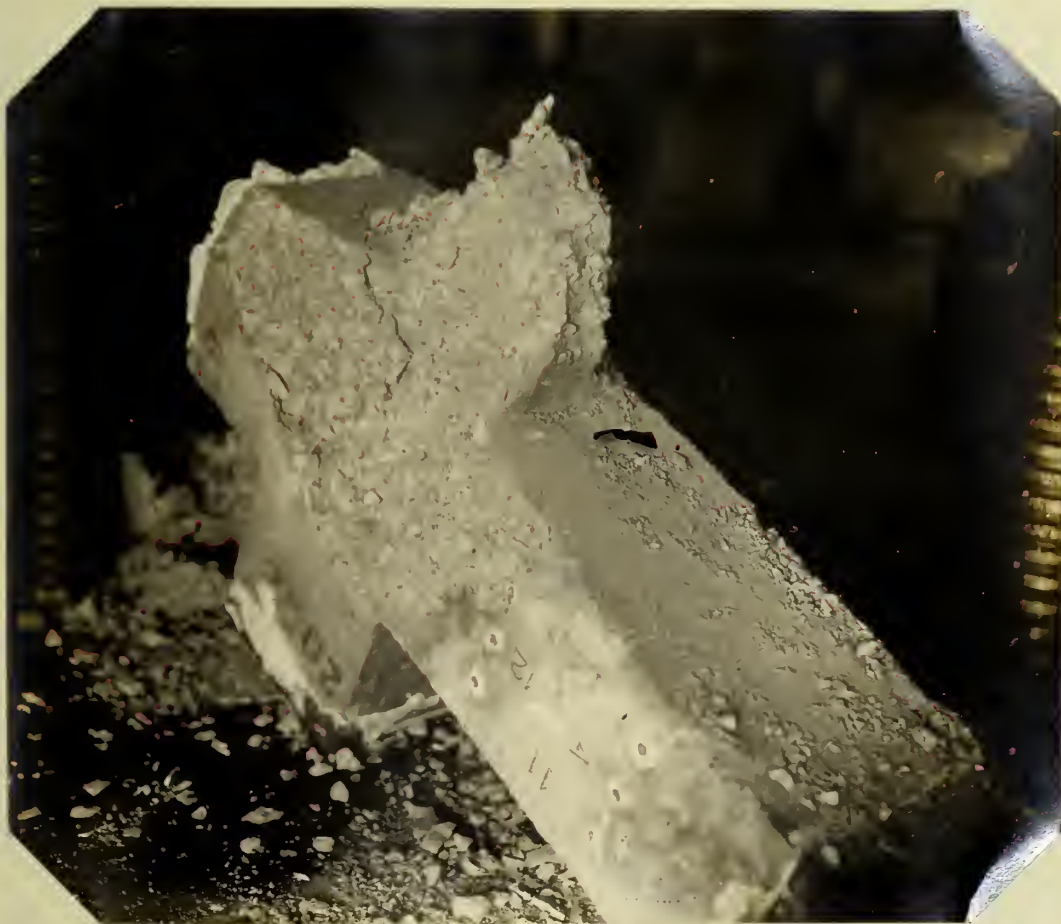
Fig. 19. Compression Specimen 2062 after Second Test.
