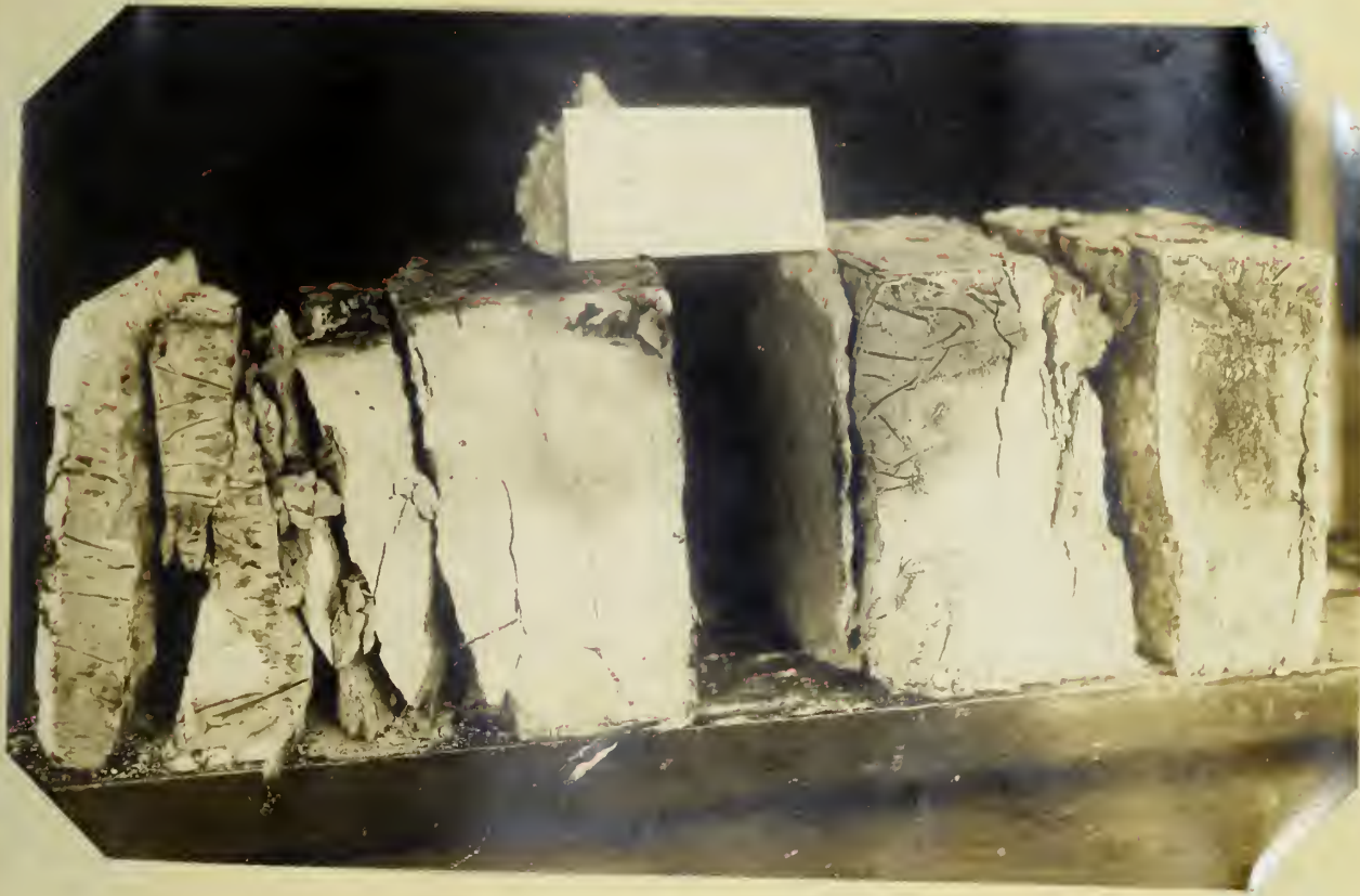
Fig. 45. 8-in. Cubes 2055 after Failure.
