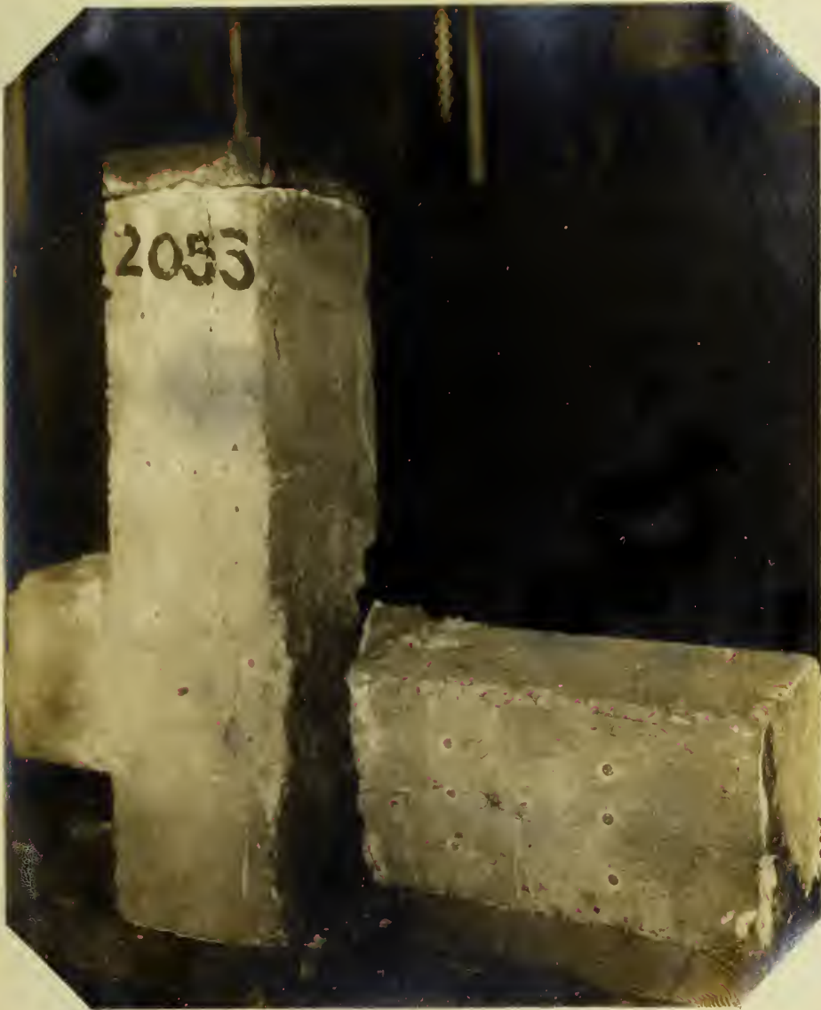
Compression Specimen 2053 after Failure.
