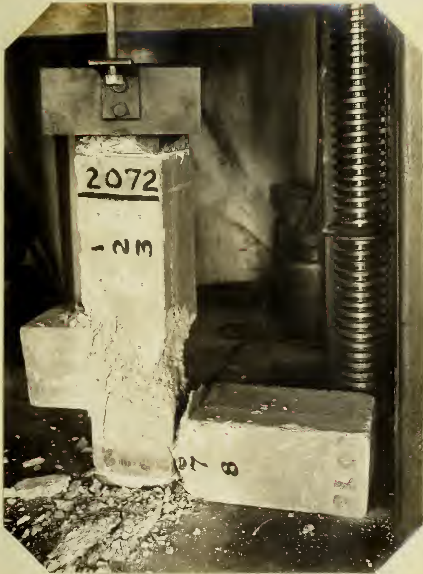
Fig. 21. Compression Specimen 2072 after Failure.
