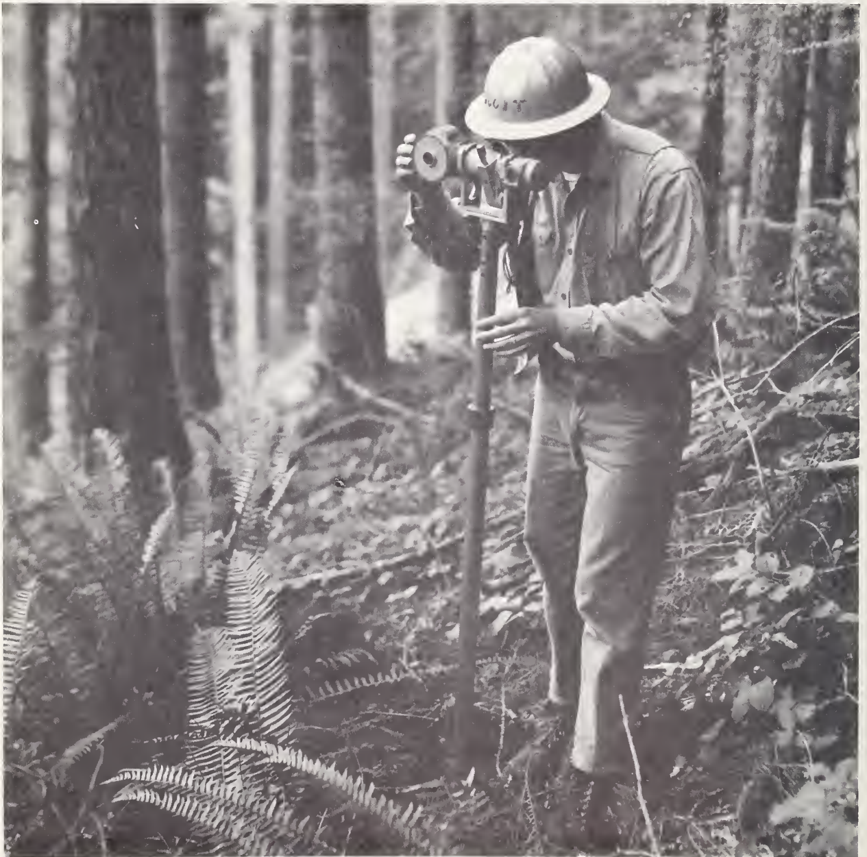
Figure 4.--Optical dendrometer used to measure upper-stem diameters and heights on standing trees.
