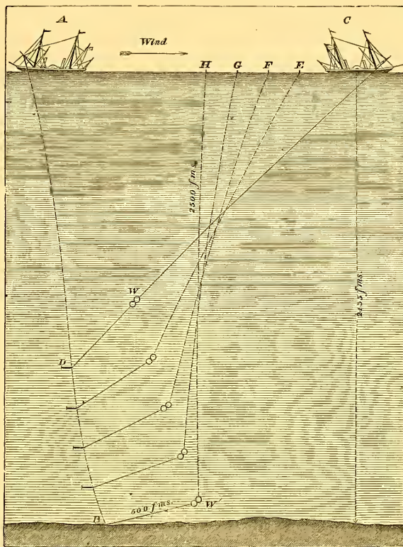
FIG. 6.—The relative positions of the Ship, the Weights, and the Dredge, at different stages of "Paying-out" from the PORCUPINE.
