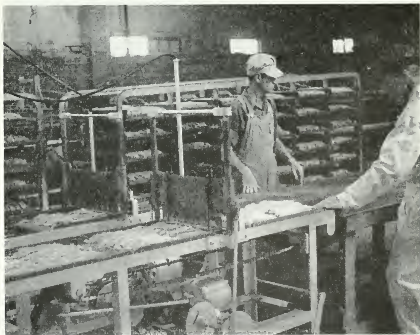
FIG. 92. Slicing the meat. The racks in the background hold meat already sliced, the method employed in this plant being to run the racks between the packing lines where they are unloaded as needed by the workers. Note the State inspector at the right.
