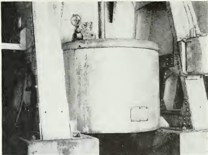
FIG. 138. The bulk centrifuge. The motor shaft is between the uprights. The skimming nozzle and its adjusting device are attached to the outer shell of the basket. Photograph by S. Ross Hatton.
