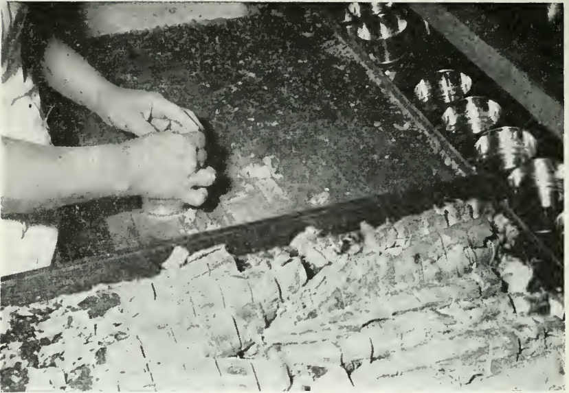
FIG. 94. Packing the tins. When filled, they are placed on the shelf seen in the upper right corner where they remain until checked by the forelady.
