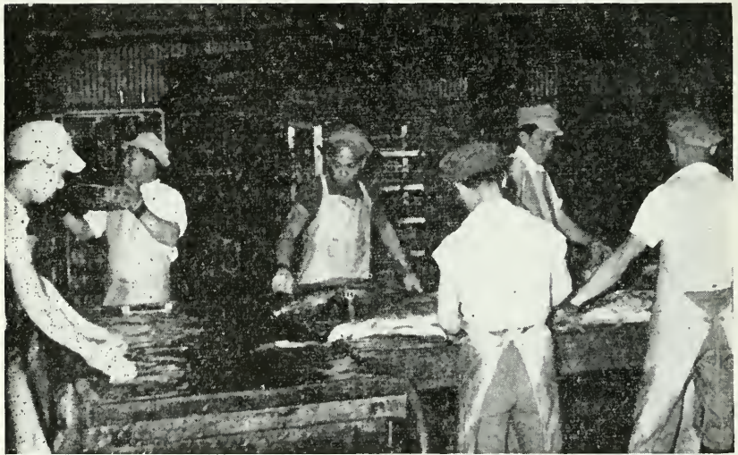
FIG. 88. Butchering yellowfin. The butchers slide the eviscerated fish into the tub where they are washed by the man at the left. The man in the left background racks the fish preparatory to the steam cook. Note the filled carriers in the background.
