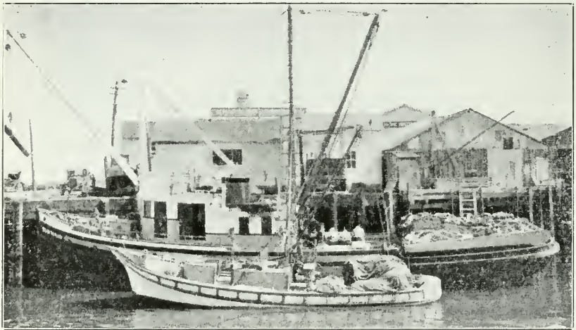
FIG. 75. Sardine boats: foreground, a Monterey lampara launch which was typical of the sardine fishing boat at that port only a few years ago; background, a purse seine boat typical of the modern sardine fleet. Photograph by J. B. Phillips, October, 1930.
