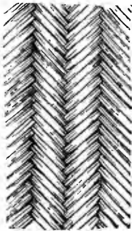
FIG. 130. DIAGONAL COMBINATION, GIVING HERRING BONE EFFECT.
