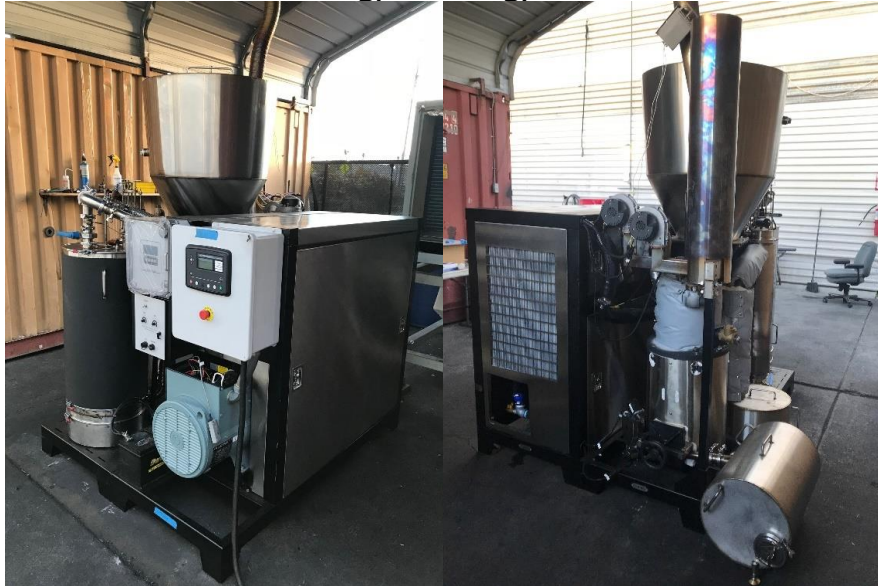
Figure 17: Final Combined Cooling, Heating, and Power Power-Pallet PP1103
