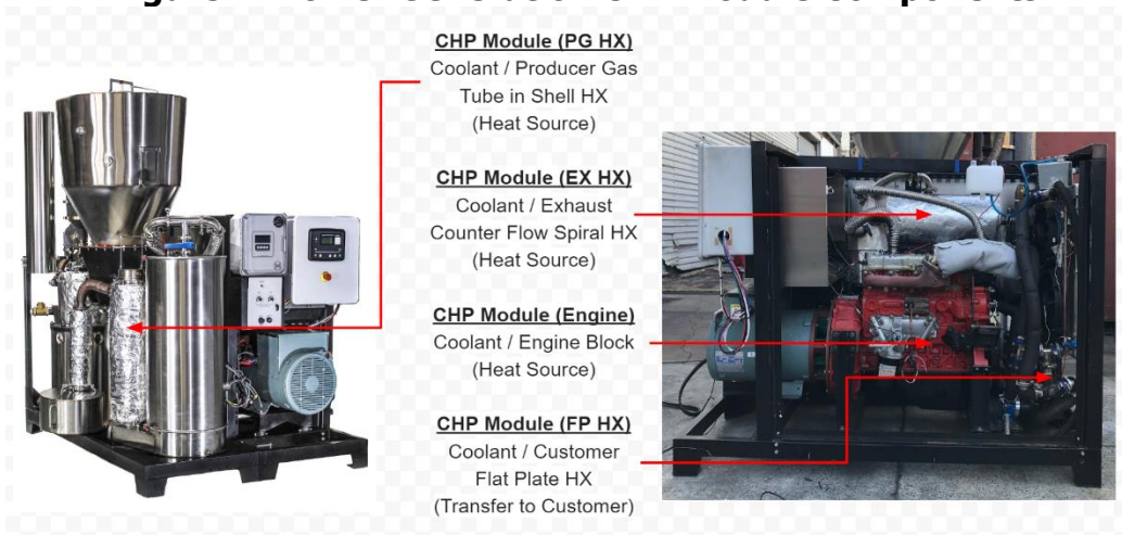
Figure 7: Power Generation CHP Module Components
