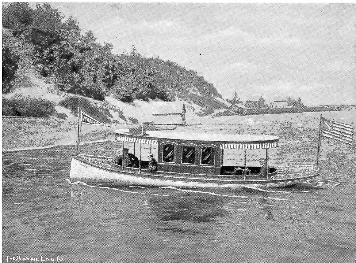
No. 5. 30 Feet. 7 Feet Beam. Six Horse Power Engine.
