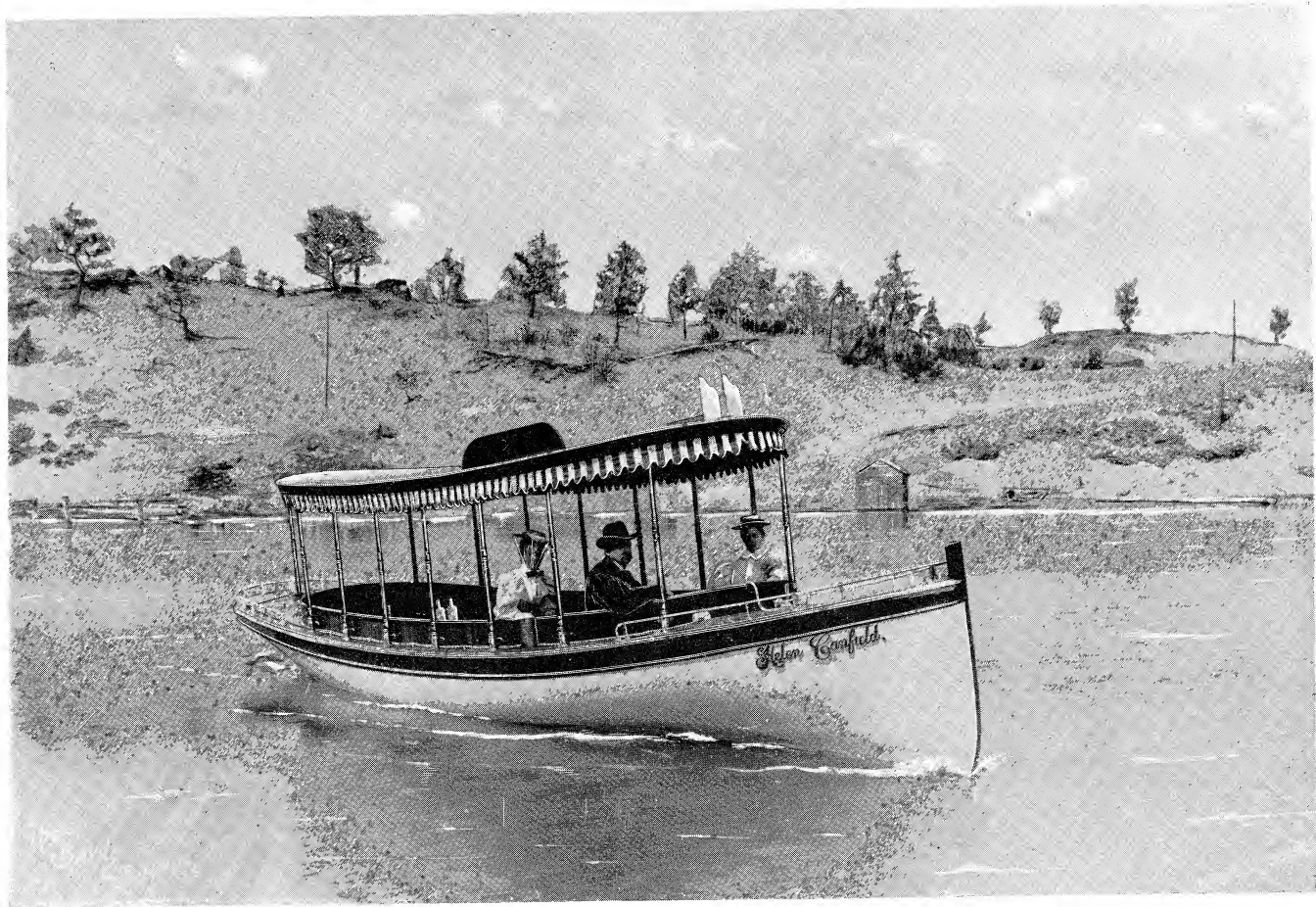
No. 4. 30 Feet Beam. Six Horse Power Engine.
