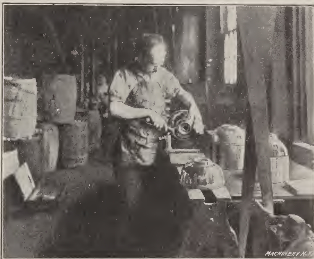
Fig. 1. View showing Method of Moistening Work with Finger Pads and also Position and Angle of Burnishing Tool
