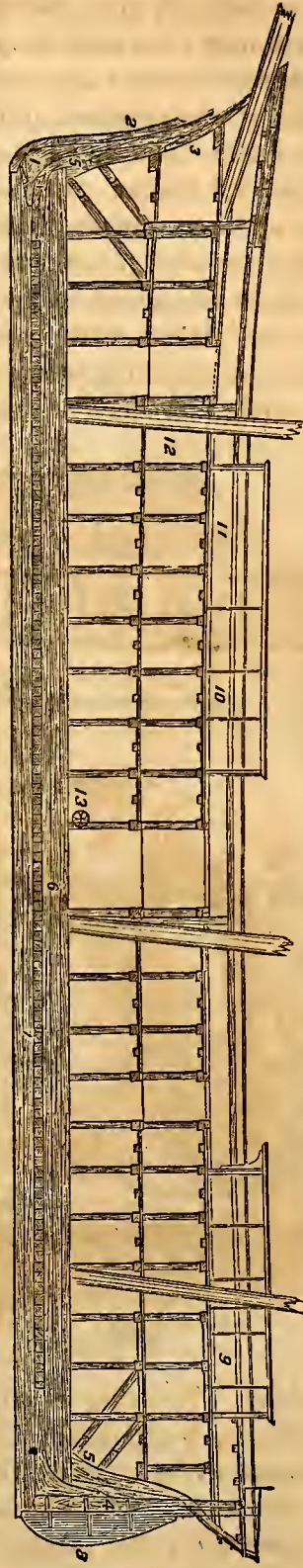
Profile Plan (showing the ship as if sawed through the centre, from stem to stern).
