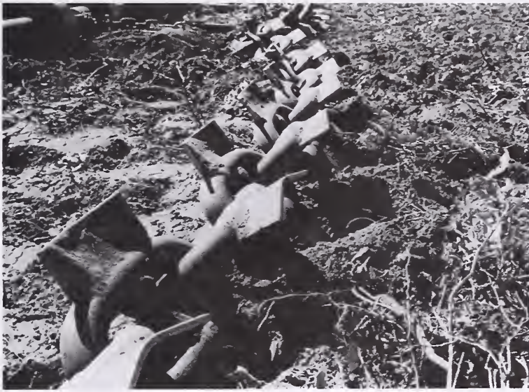
Figure 1 —Disk-chain-diker implement under development by the Texas Agricultural Experiment Station for enhanced seedbed preparation on debris-littered rangeland. The combination of the disk chain (front portion of implement) and chain diker (rear portion) provides tillage, land smoothing, and basin formation in a single pass.
