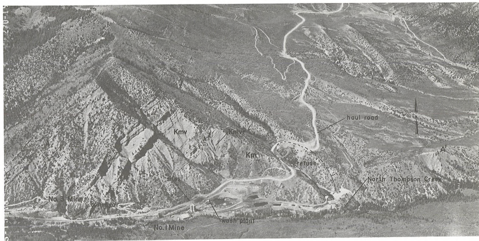
Figure A1-1. Looking north at the North Thompson Creek No. 1 and No. 3 mines. Currently, the coal is hauled by truck approximately 13 miles to rail loadout facilities at Carbondale, Colorado. Kmv indicates the coal bearing Mesaverde formation, Kmvr the Rollins sandstone member of the Mesaverde, and Km the Mancos shale. Coal beds in the area dip at an angle of 27 to 30 degrees. The distance from A to A' is approximately 1 mile.
