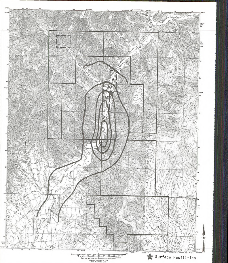
Map S3-1 Predicted increases in ambient concentrations in 1980 (micrograms per cubic meter)
