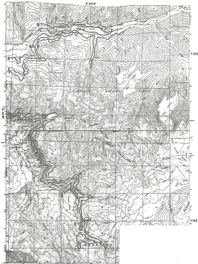
Figure AR2-3. Outcrop of the B, E, and F coal seams at the Mt. Gunnison No. 1 Mine
