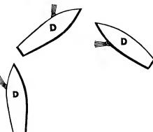
If A sees a White Mast-head Light above the Red Light, A knows that the vessel is a steam-vessel, and is either approaching her in the same direction, as B, or is crossing to port in some direction, as D D D.
