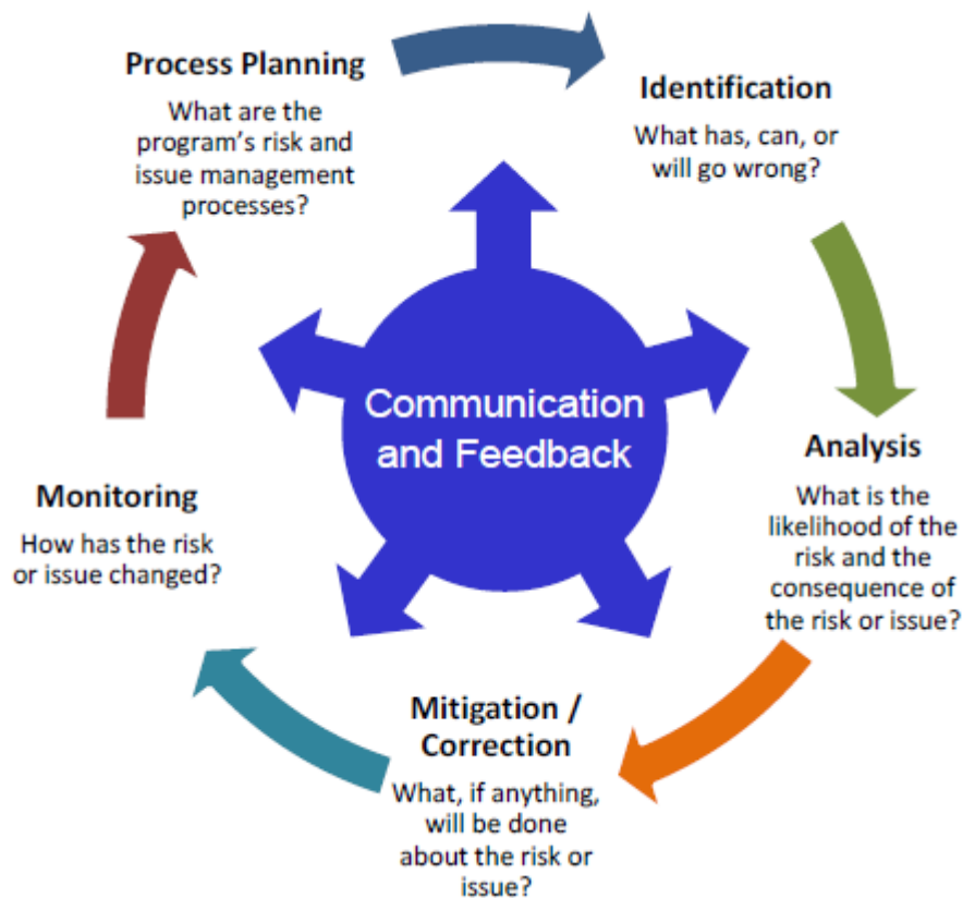
Figure 86. Risk and Issue Management Process Overview. Source: Office of the Deputy Assistant Secretary of Defense for Systems Engineering (2017).
