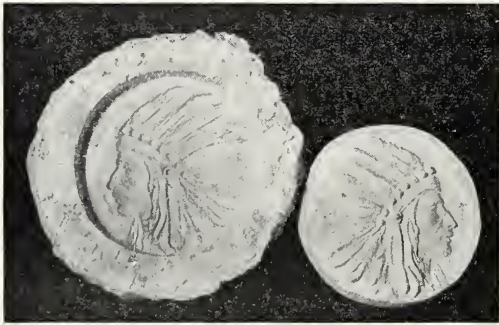
Figure V. Plaster mold and cast from wax model
