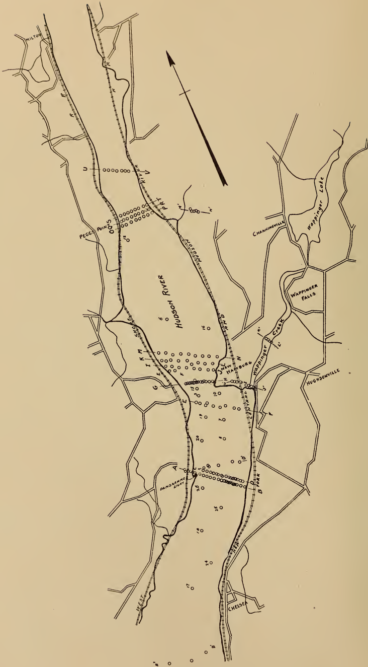
Fig. 9 Key map showing the locations of lines of wash borings forming the basis of the accompanying cross sections of the Hudson above the Highlands
