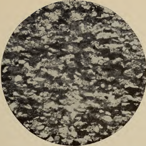
Photomicrograph showing structure of the reeding quality of "blue-stone." Magnification 30 diameters. Taken to show tendency to parallelism of elongate grains.
