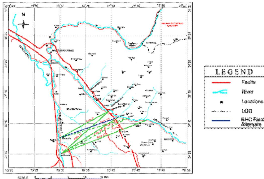
**Figure 9** Fault line passing through the reservoir of the new dam site
