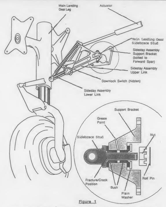
Note: This figure is provided to depict the area of the sidebrace stud to be inspected. This is not intended to represent the configuration of all models affected.
