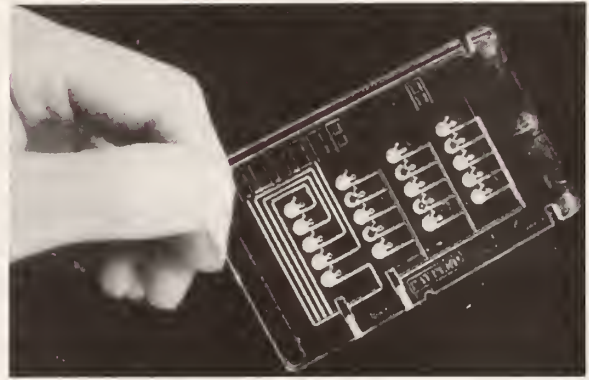
Photo of bioMerieux Vitek susceptibility testing reagent card. It was originally developed by NASA to diagnose urinary tract infections in astronauts in space and had to be very small. Courtesy of James H. Jorgensen, University of Texas Health Science Center, San Antonio, TX, 1995.
