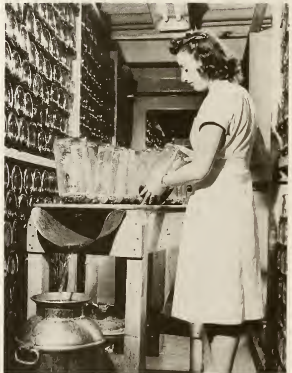
A production worker pouring penicillin-containing culture medium into a trough for collection in a milk can, mid-1940s. Photo courtesy of The National Museum of American History, Smithsonian Institution, Washington, DC.
